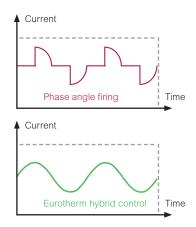
Analog thyristor controllers waste energy by drawing more power from the supply than is required by the heater, due to harmonic generation at most setpoint levels.
