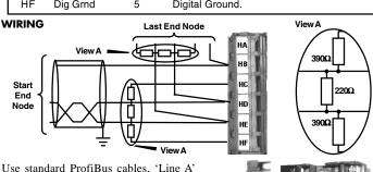
and 'Line B', with special 9 pin D Type male connector headers, allowing one or two cables to be fitted. A termination load is built in with an ON/OFF switch. set to ON at the two ends of the line. When using 9 pin D Type connections a further assembly is required.
