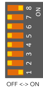
Example shows 4 wire and address 1
