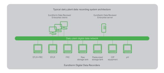
A typical pasteurization data collection system uses a secured, isolated, and remote PC/server for archiving data related to thermal and flow limit devices. From this PC/server, the Eurotherm Data Reviewer software allows for inspection, audit, analysis, approval, exporting, and printing of data and metadata related to the milk pasteurization process.
