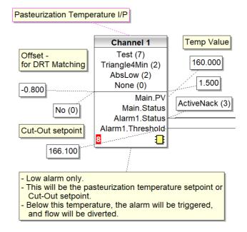
For the Eurotherm standardized 6100A and 6180A STLR and FRC public health control solutions a table-based configuration is used. Although this can be provided as a printout, configuration information is more easily reviewed using Eurotherm C-Edit software. C-Edit software can be downloaded for free as part of the 6000 Series Tools software package www.eurotherm.com/6000.
