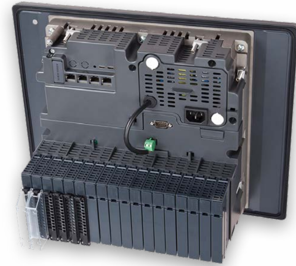
EPM-15 - 15" widescreen model, 18 I/O module slots Up to 54 high precision AI channels onboard
