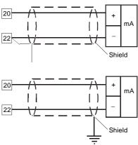
Fig. 6.A mA INPUT WIRING
