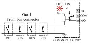
Fig. 20/B Relay energized, beacon OFF lit.
