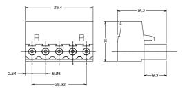
Fig. 24 - 5 wires connector
