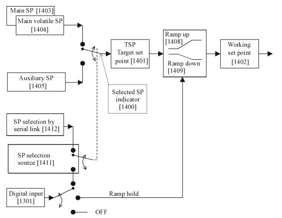
NOTE: the main SP (1403) is a value memorized in EEPROM while the main volatile SP (1404) is a value memorized in RAM. For this reason, when you make a profile setting the set point value by serial link (e.g. with a supervisory system), it is advisable to use the main volatile SP, instead of the main SP (the EEPROM has a limited number of write actions allowed while the RAM has no limit).
