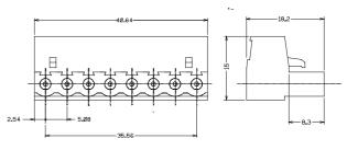
Fig. 25 - 8 wires connector
