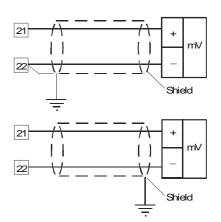
Fig. 6.B 60mV INPUT WIRING
