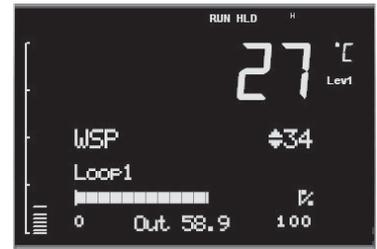
WSP is the Working Setpoint and is the current setpoint derived from the programmer. To change the value of WSP the programmer must be put into Hold, then it can be adjusted using the
