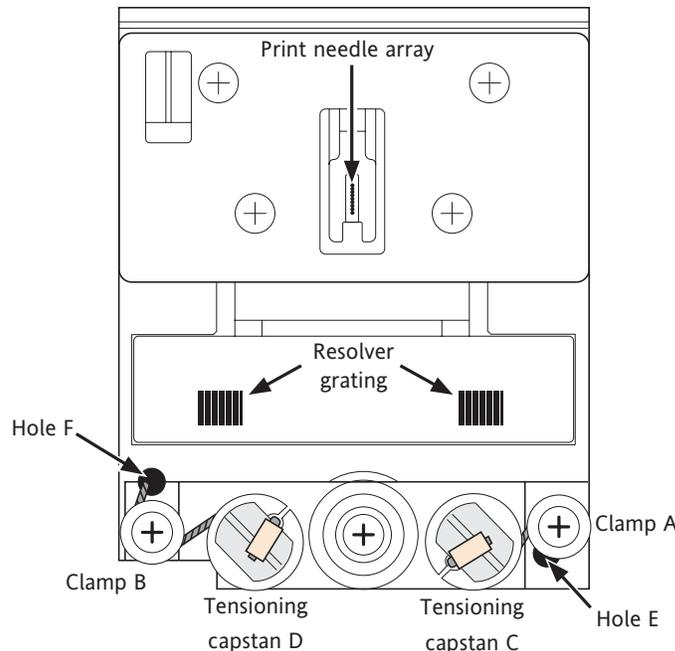
Figure 5.4.6a Print head carriage assembly (front view)
