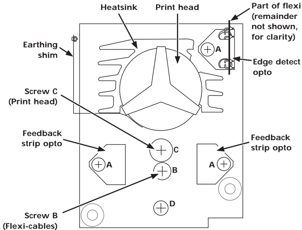
Figure 5.2.2 Print head carriage assembly - component locations
