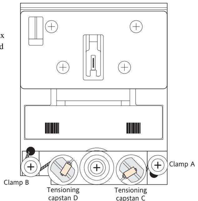
Figure 5.4.8 Cord tension components
