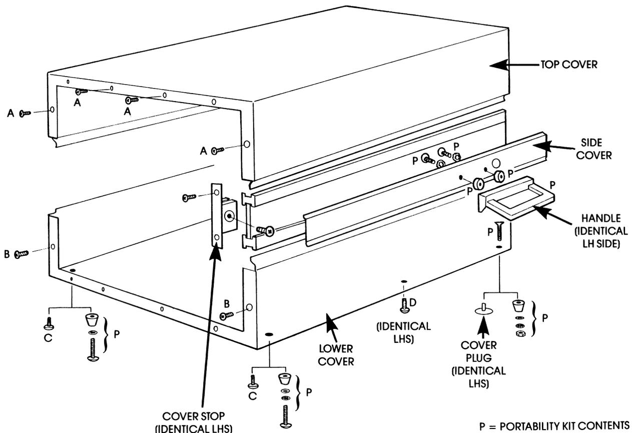
Figure 5.10 Case - exploded diagram (Rear view)
