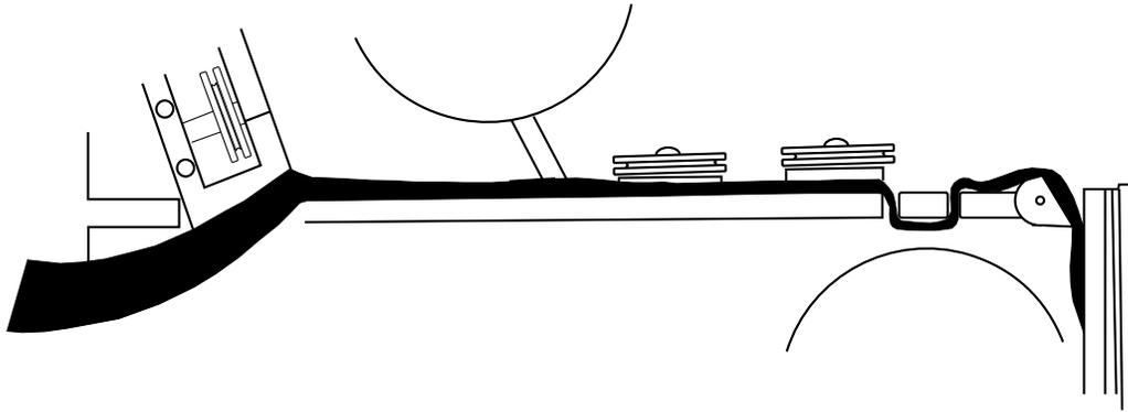
Figure 5.8.3 Chart control harness routing
