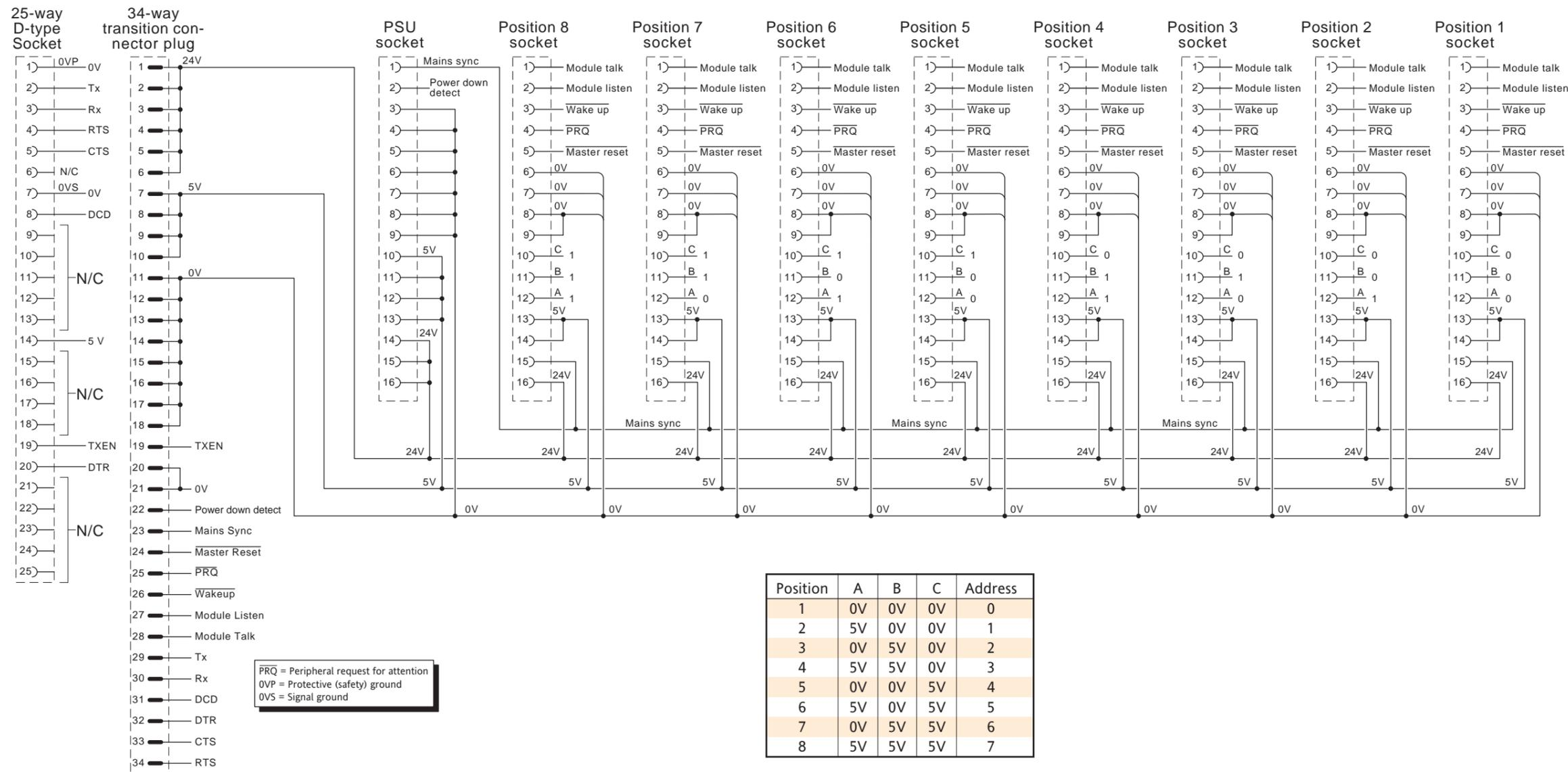
Figure 6.5.1 Mother board schematic
