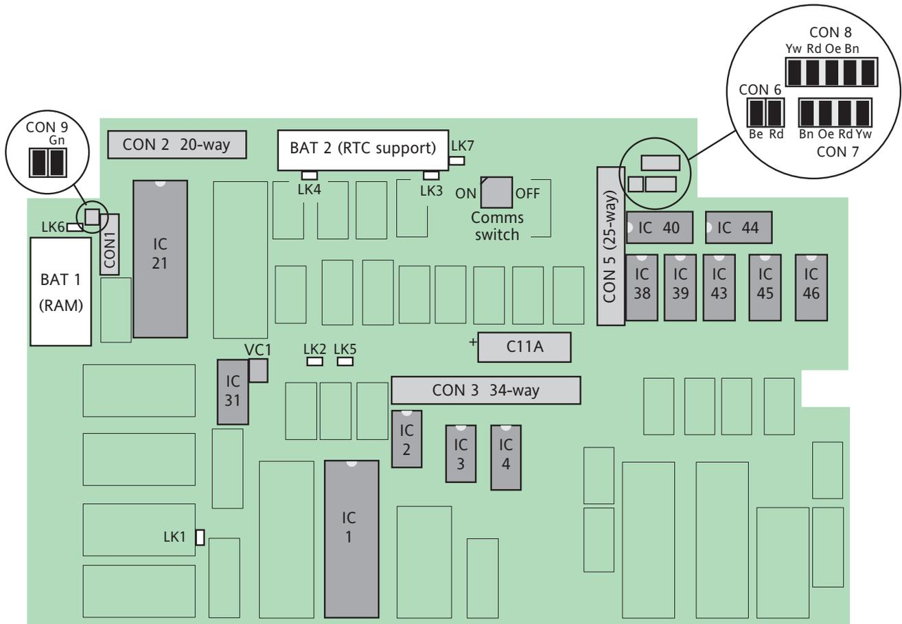
Figure 3.8a Control board connector and link positions (Mark I control board)
