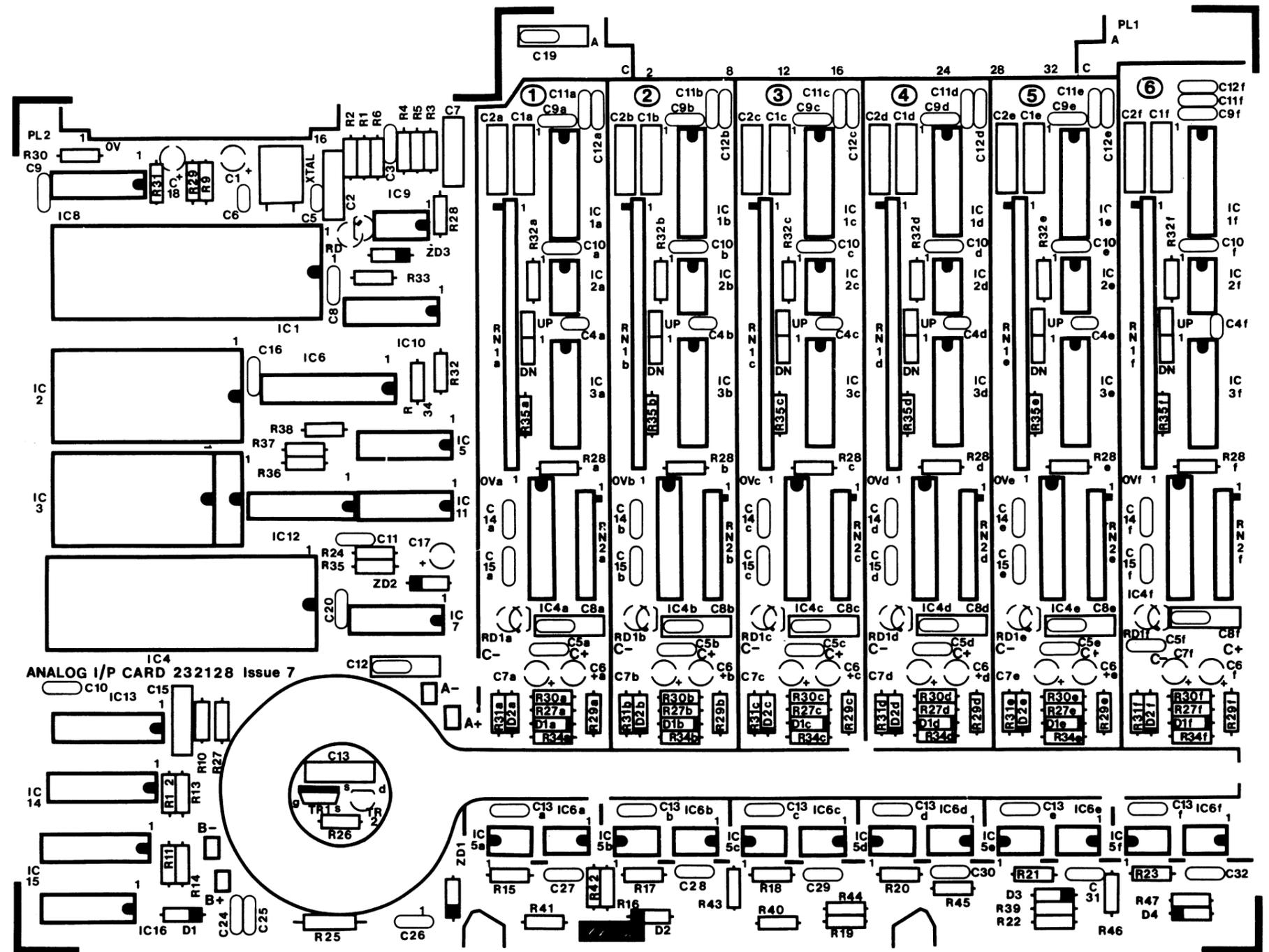
Figure 6.1.1 DC input board component layout
