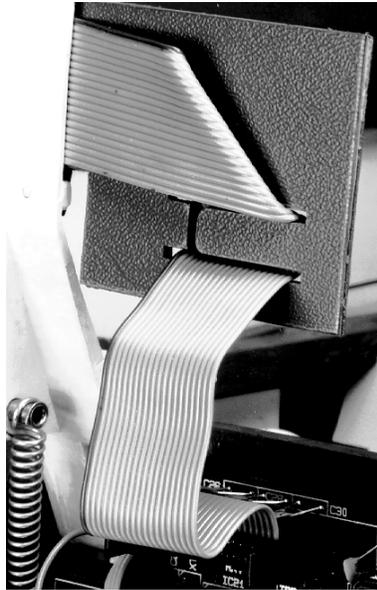
Figure 5.9.3 Ribbon cable retaining bracket
