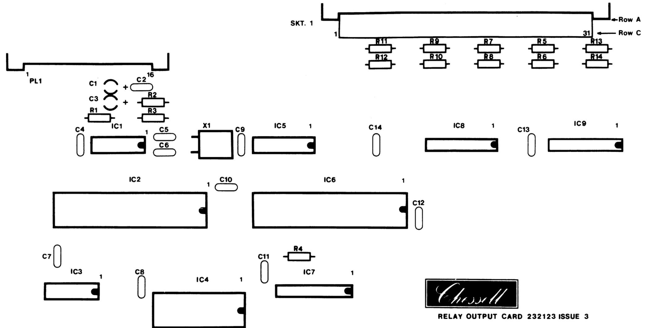
Figure 6.6.1 Relay output board component layout
