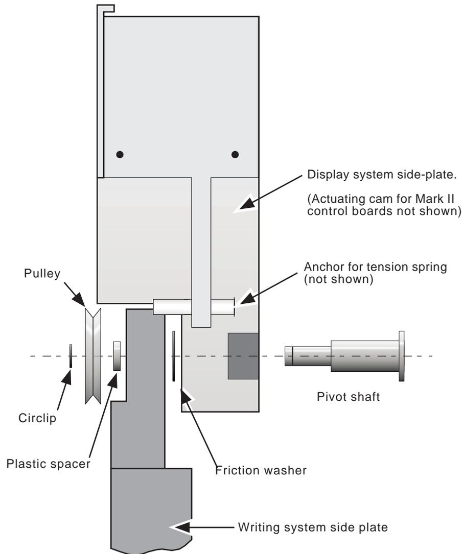
Figure 5.5.16 Right-hand pivot assembly (rear view). Left-hand similar.
