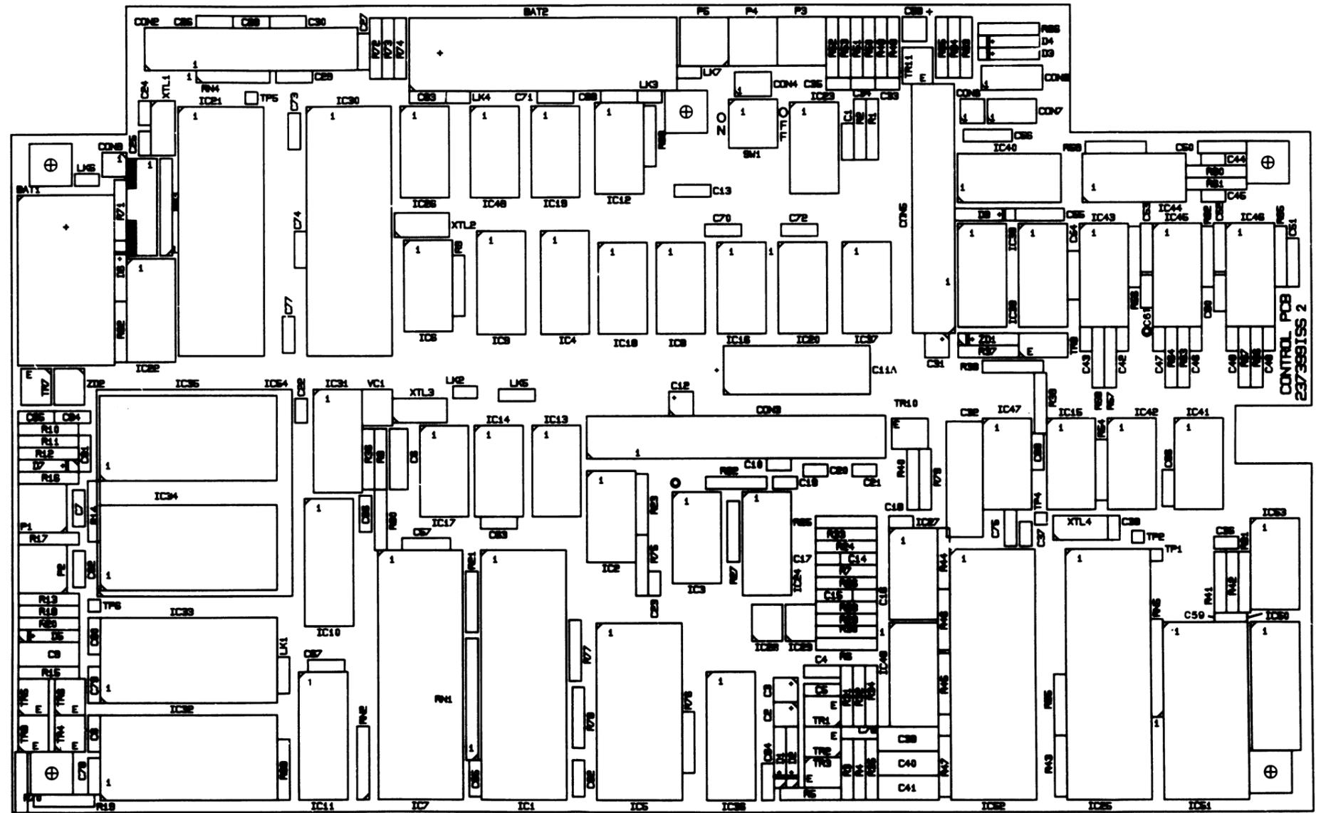
Figure 6.3.2 Mark I Control board layout
