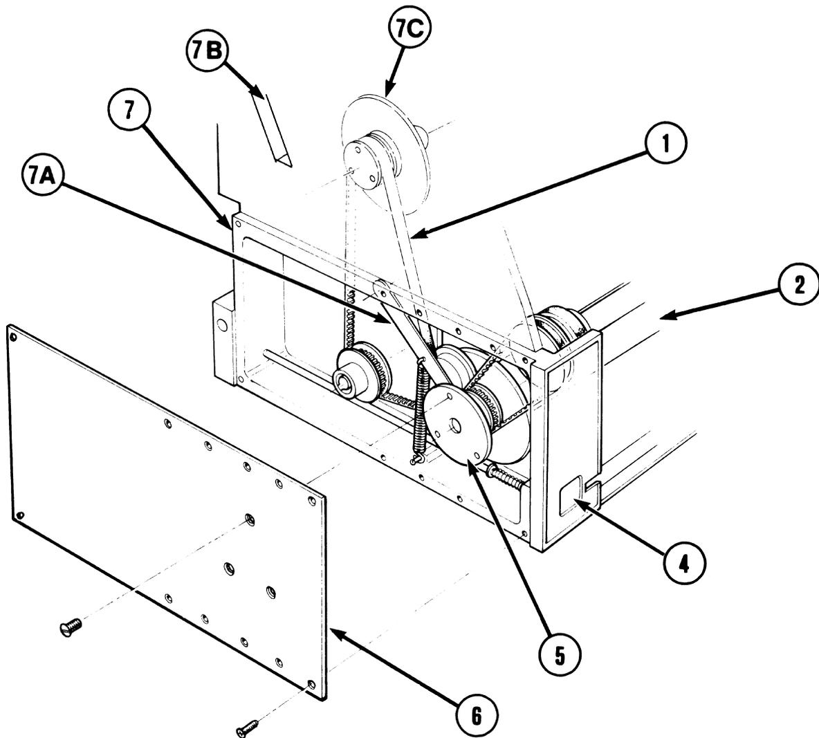
Figure 8.5 Exploded diagram: Chart drive system sheet 1 of 2
