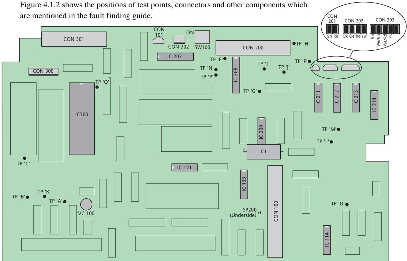
Figure 4.1.2 mark II control board component locations
