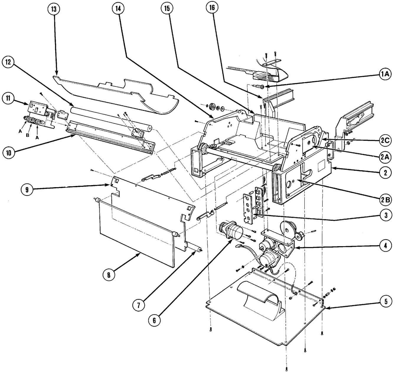
Figure 8.4 Exploded diagram: Writing system (original design) sheet 1 of 2
