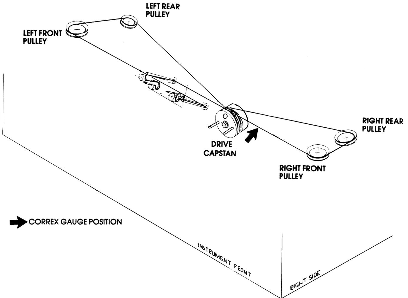
Figure 5.4.6d Print head carriage cord routing
