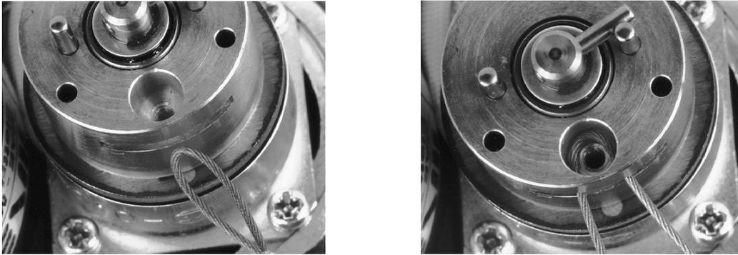
Figure 5.4.6b Drive capstan cord clamping
