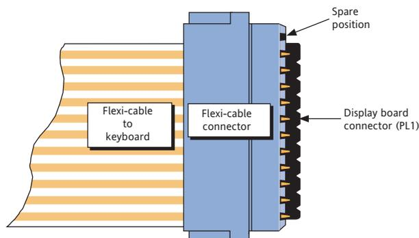
Figure 5.9.4 Keyboard flexi connector location
