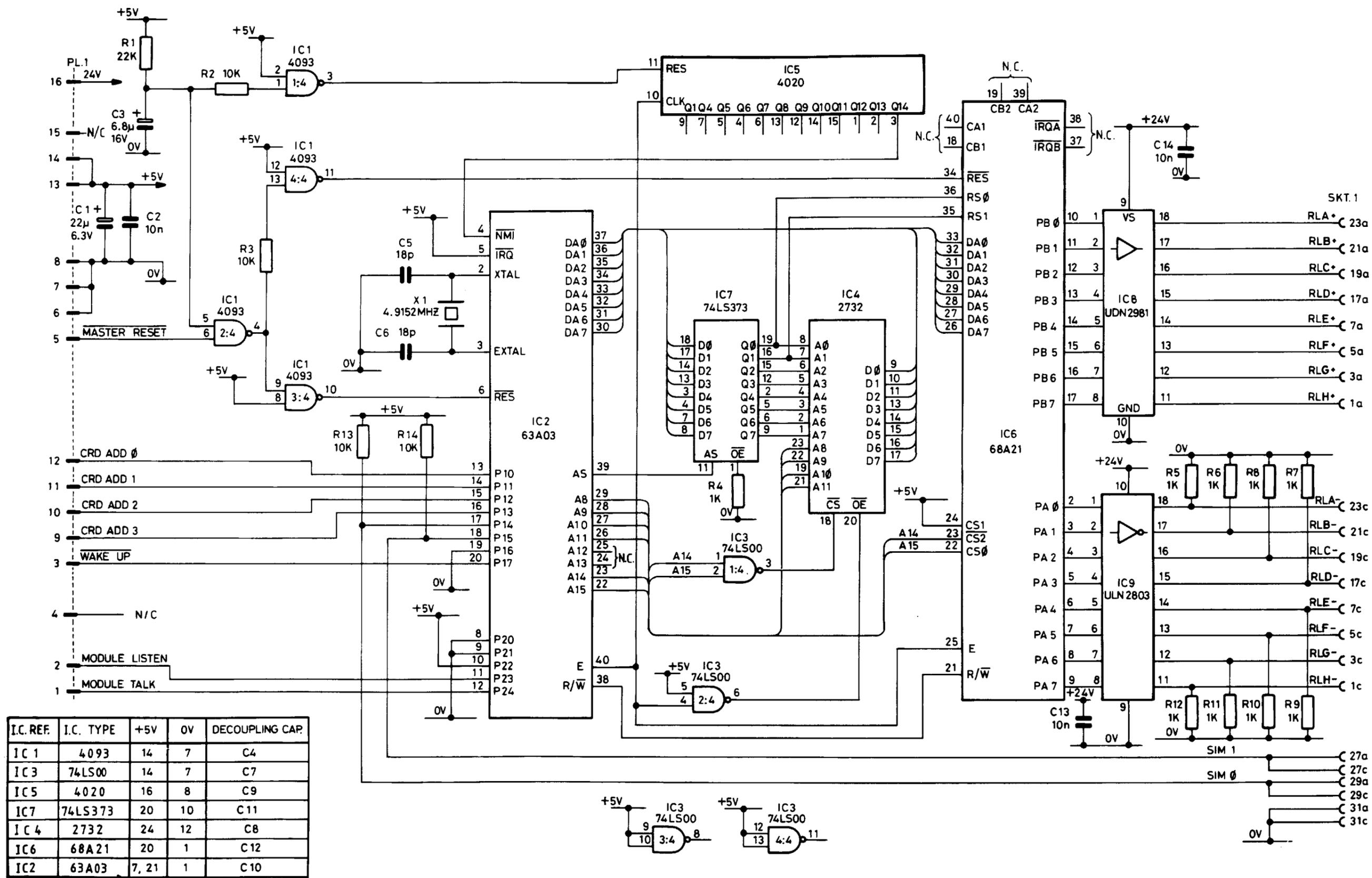
Figure 6.6.2 Relay output board schematic
