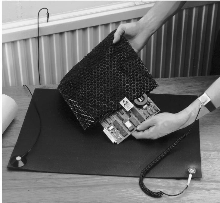
Figure 5.1.1 Typical static prevention kit
