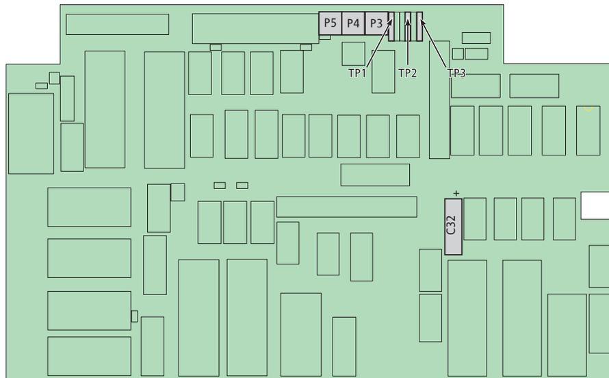
Figure 5.5.1a Potentiometers and test points on the Mark I control board
