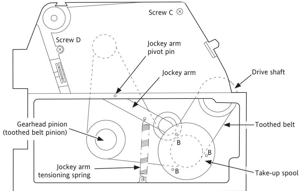
Figure 5.7 Chart drive arrangement (cover plate removed)
