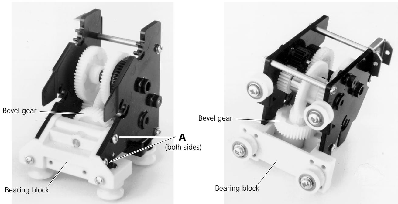
Figure 5.3.3 Ribbon cartridge carriage gearbox (two views)
