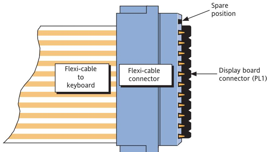
Figure 5.11.4b Keyboard flexi connector detail
