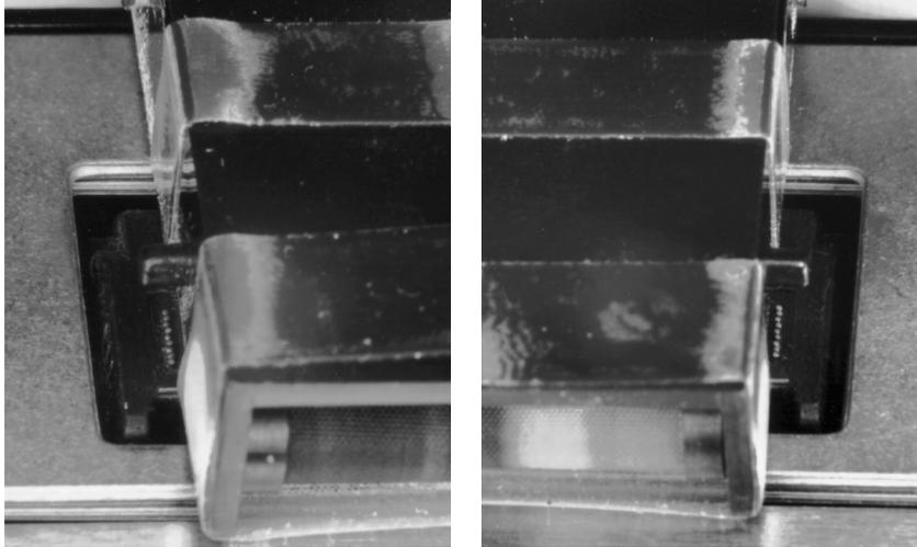
Figure 5.4.9 Print needle array location *versus* ribbon cartridge edge
