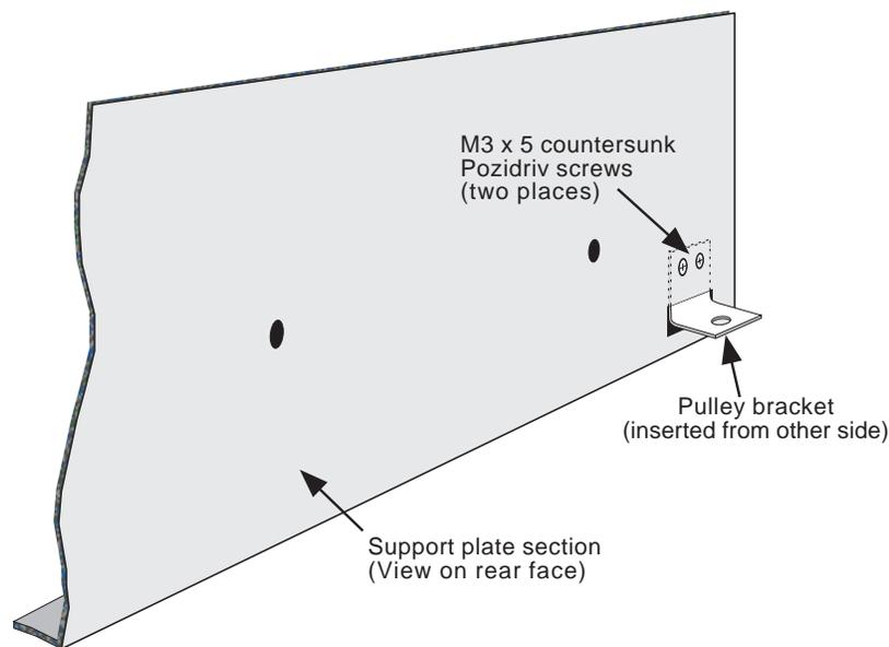
Figure 5.15.5a Pulley bracket fixing
