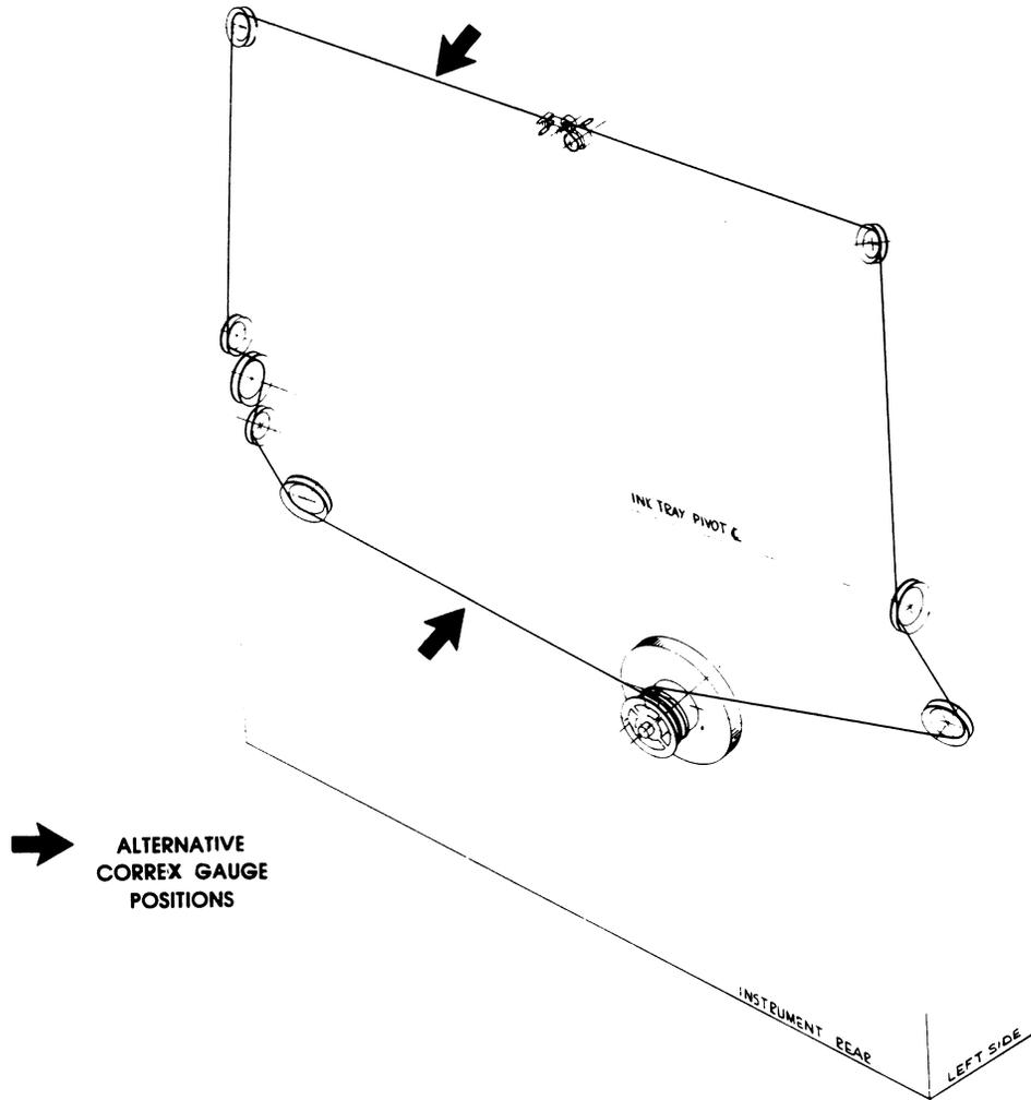
Figure 5.4.7a Ribbon cartridge cording
