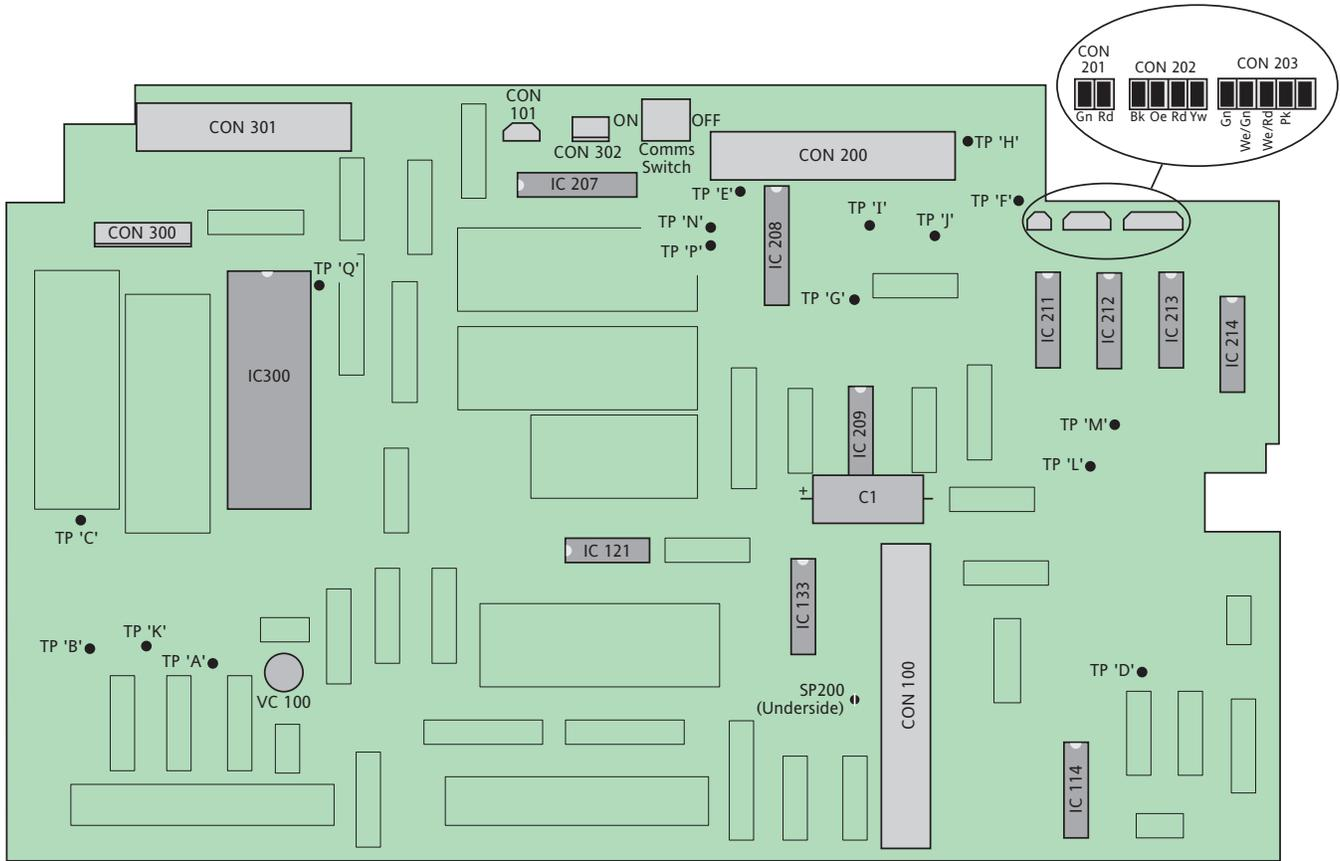
Figure 3.8b Control board connector and test-point positions (MarkII control board)
