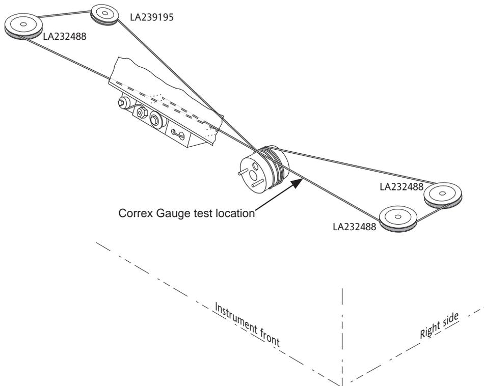
Figure 5.4.4a Print head carriage cord routing
