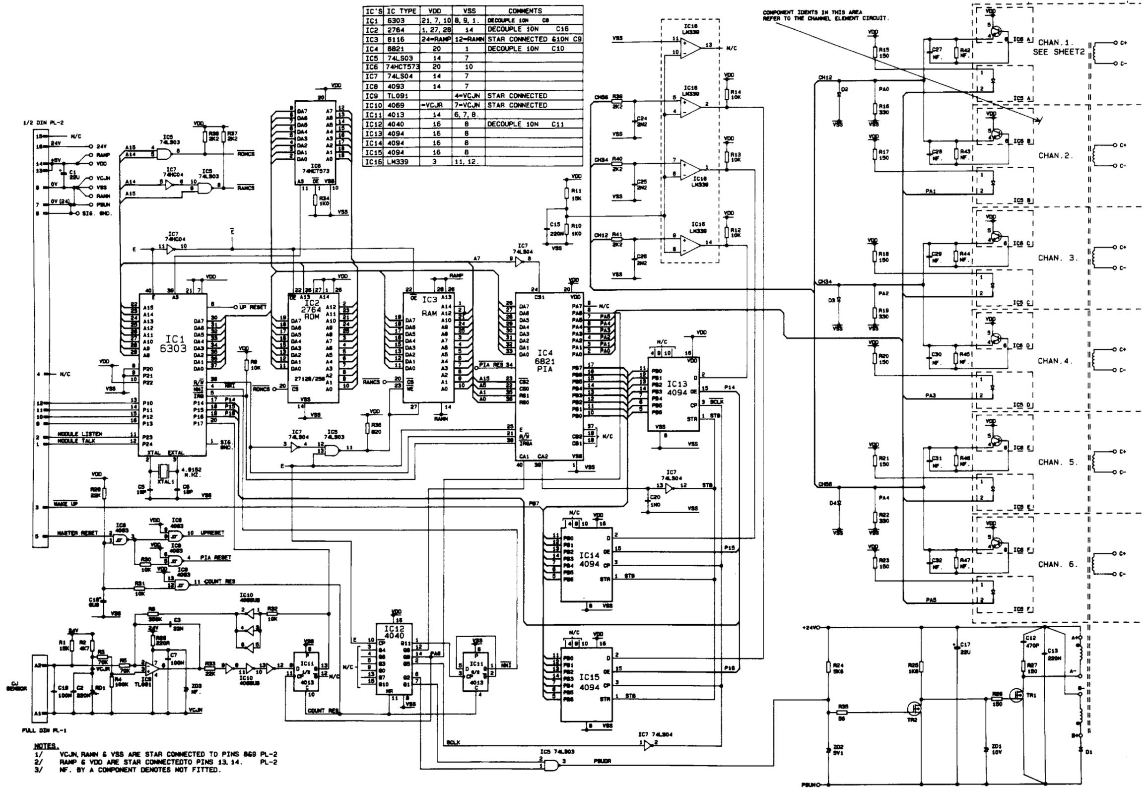
Figure 6.1.2a DC input board schematic (sheet 1)
