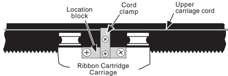
Figure 5.4.5b View on underside of the ribbon cartridge carriage.
