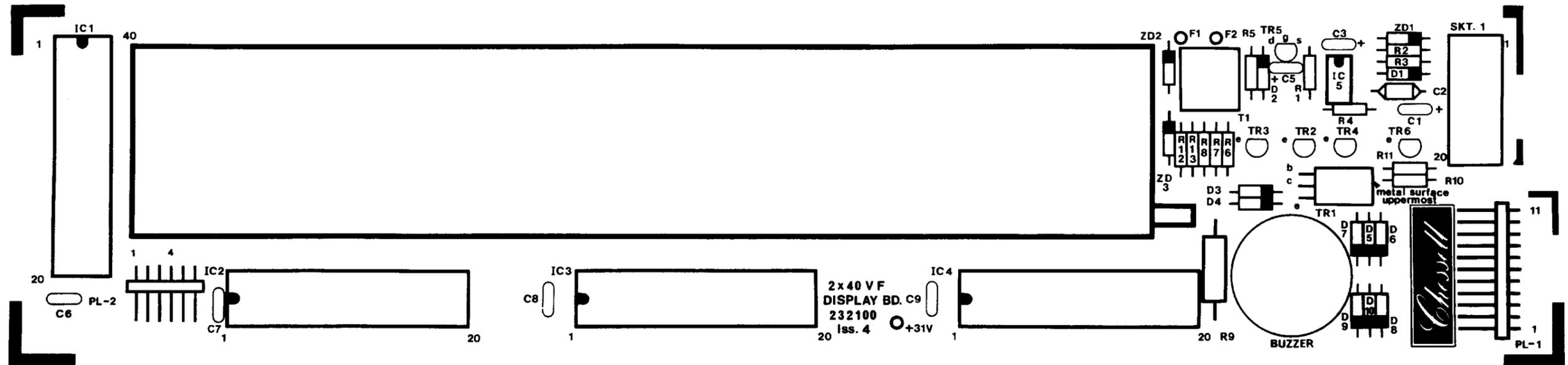
Figure 6.7.1 Display board component layout
