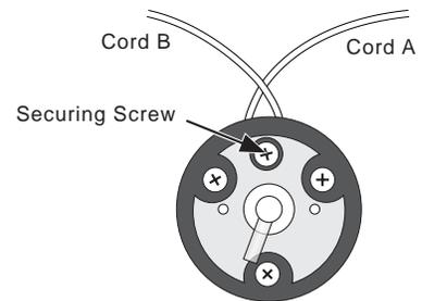
Fig 5.4.4b Cord securing detail
