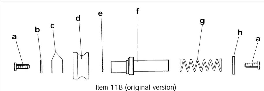
Figure 8.4 Exploded diagram: Writing system (original design) sheet 2 of 2
