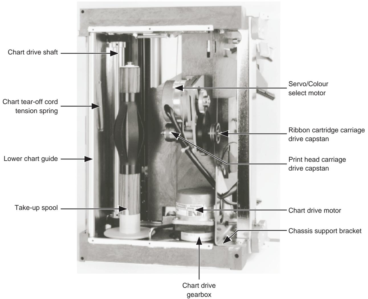
Figure 1.1.1c Writing system view on underside
