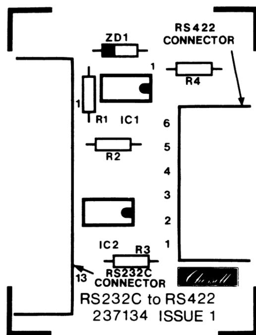
Figure 6.8.1 Conversion module component layout
