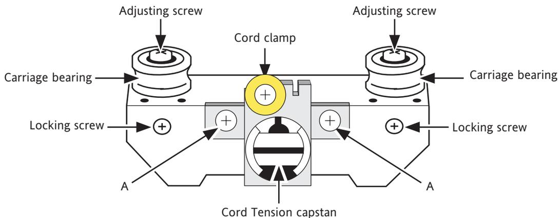
Figure 5.3.2 Ribbon cartridge carriage adjustment
