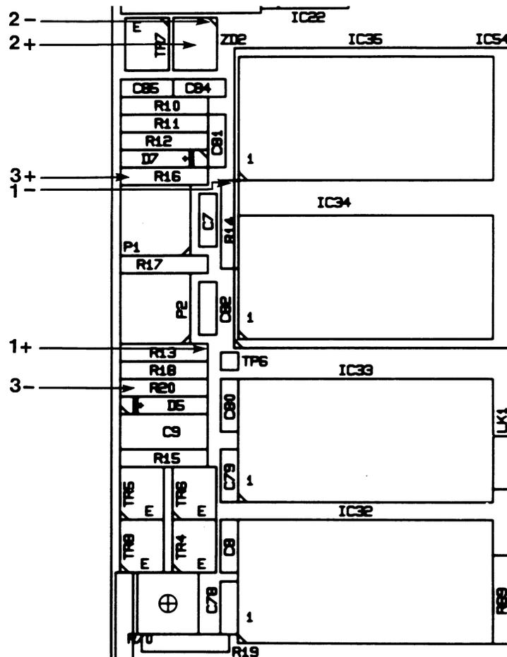
Figure 6.3.1 Control board measuring points
