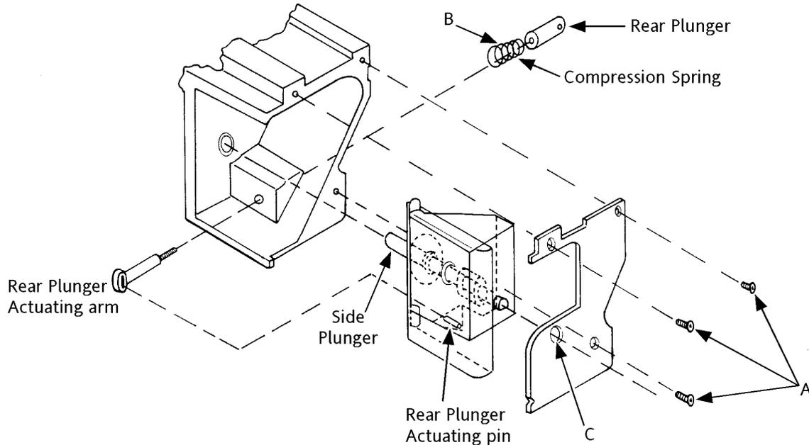
Figure 5.11.4a Left hand catch assembly (right hand similar)
