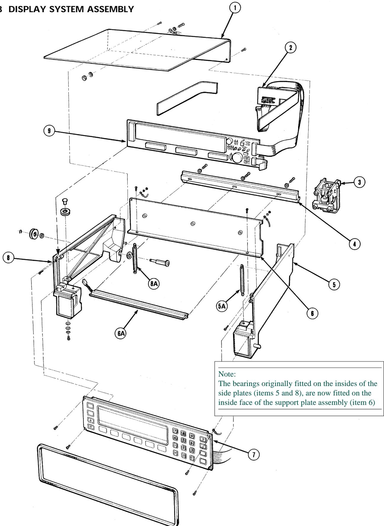
Figure 8.3 Exploded diagram: Display system (original design)
