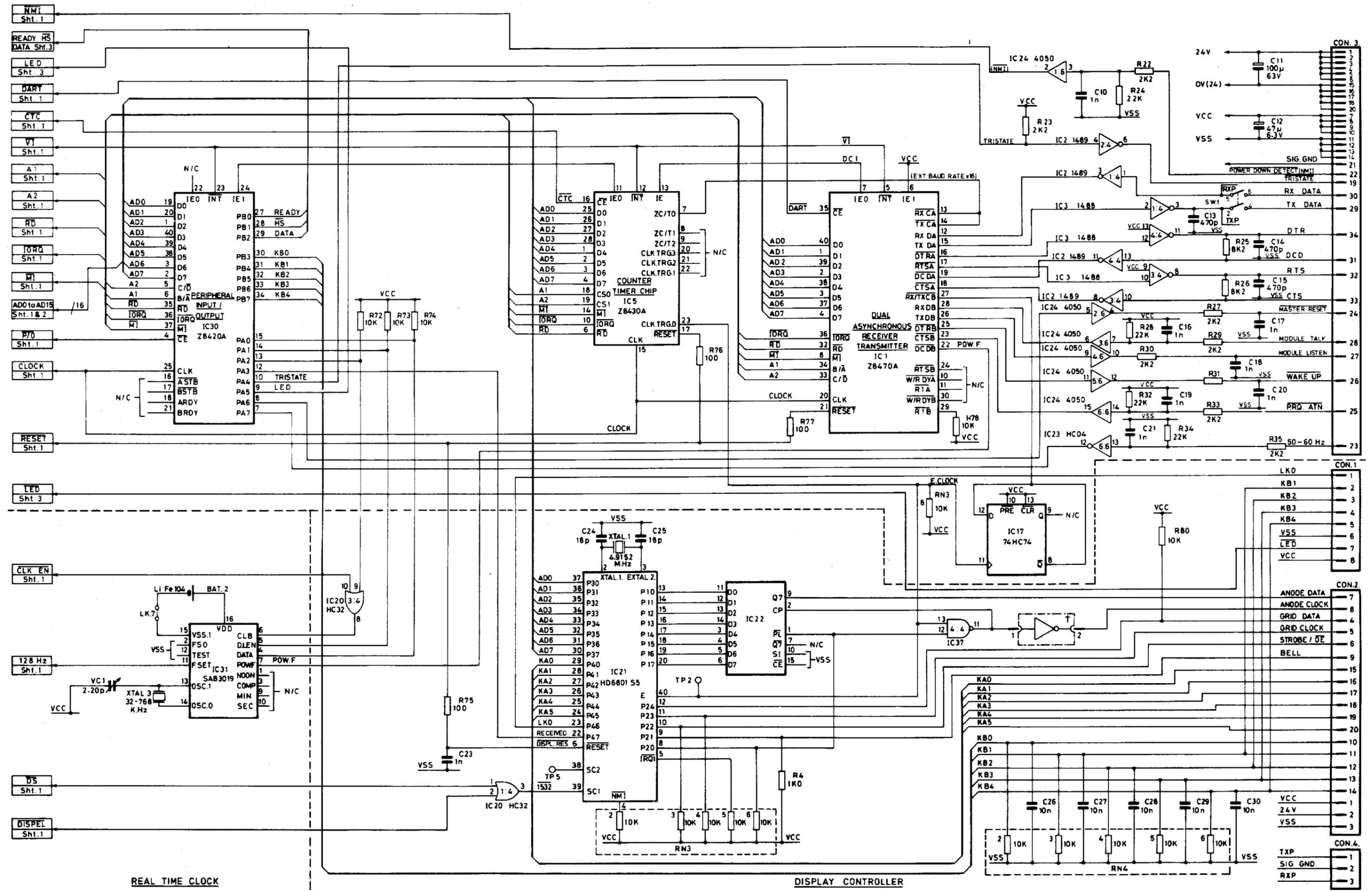
Figure 6.3.3b Mark I Control board schematic (sheet 2)
