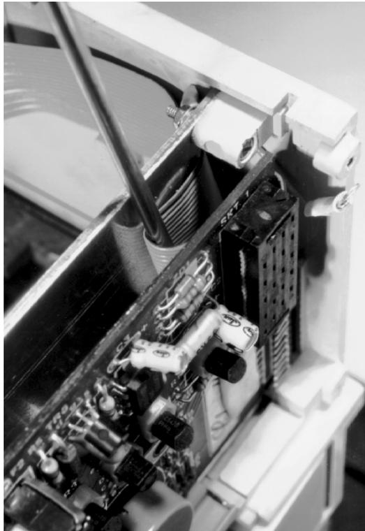
Figure 5.14.2a Ribbon cable manipulation
