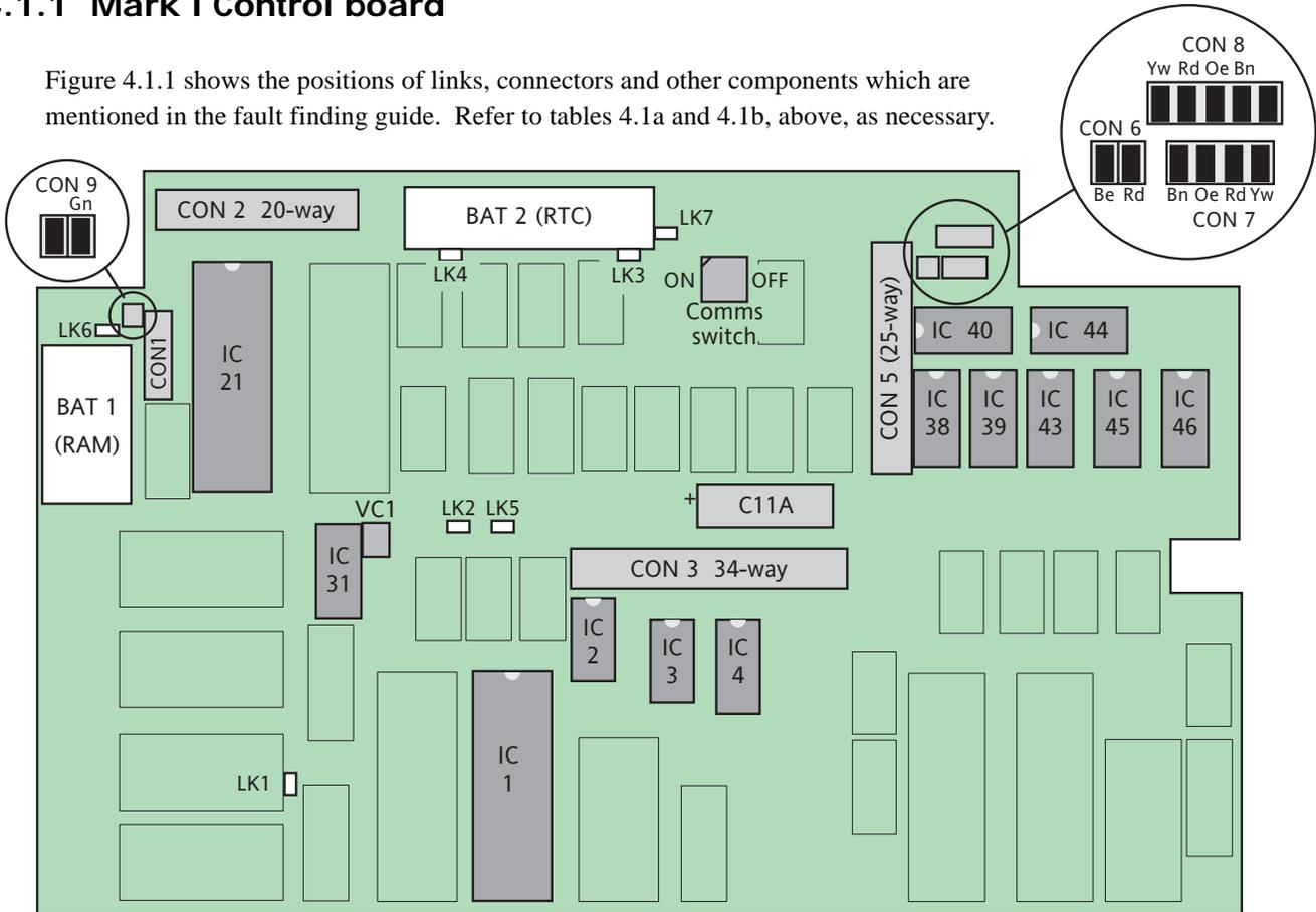
Figure 4.1.1 Component locations (Mark 1 Control board)
