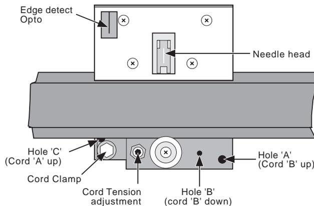
Figure 5.4.4c Print head carriage cord clamping
