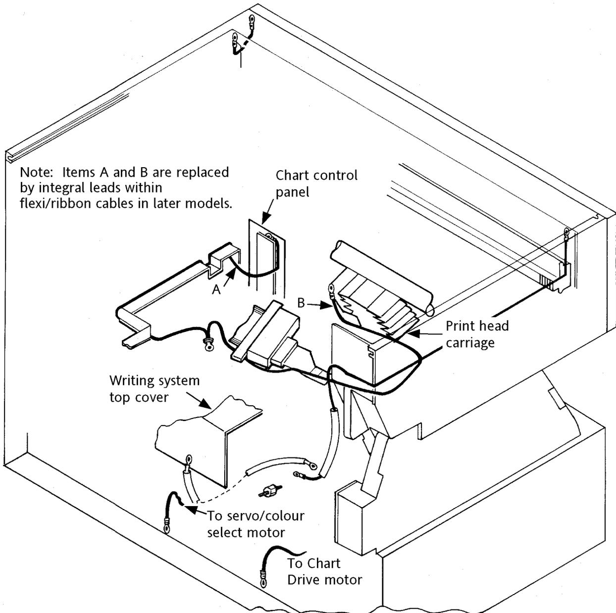
Figure 5.12.1a Grounding wire arrangement
