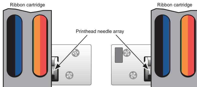
Figure 5.4.5d Checking the ribbon cartridge is central with respect to the print head needles
