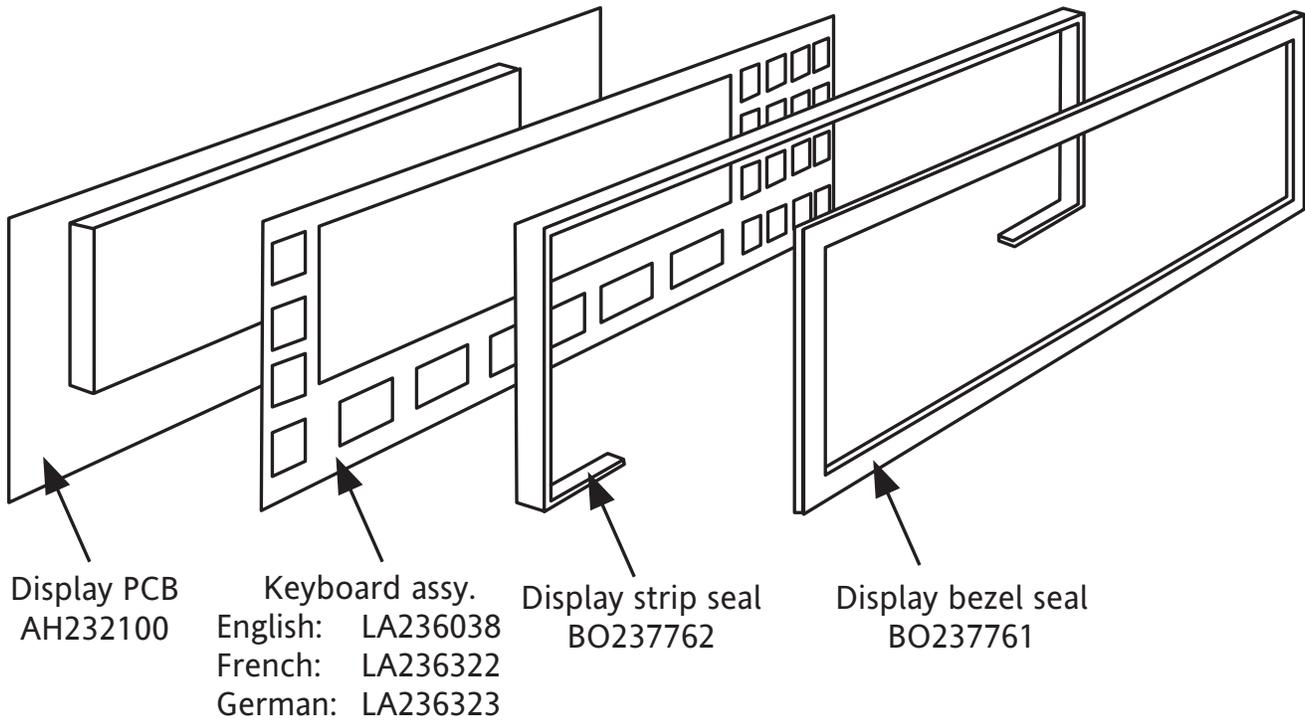
Figure 7.14.2b Writing system spares (display unit)
