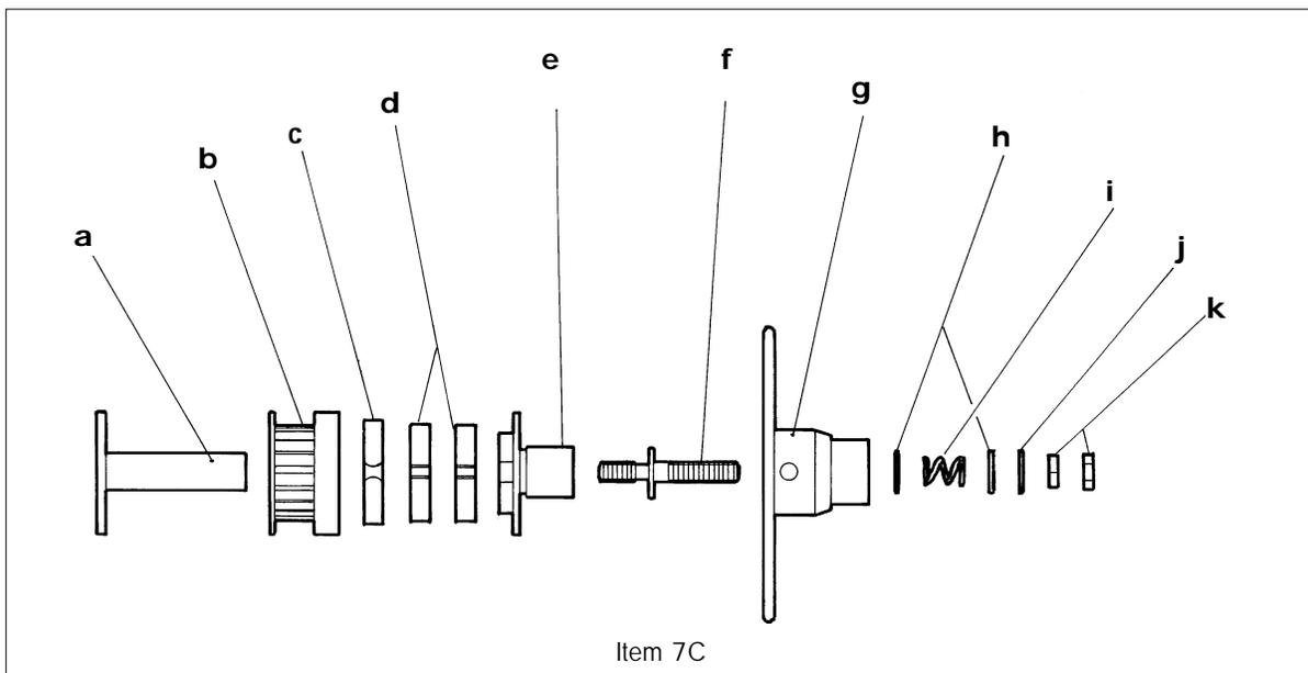
Figure 8.5 Exploded diagram: Chart drive system sheet 2 of 2
