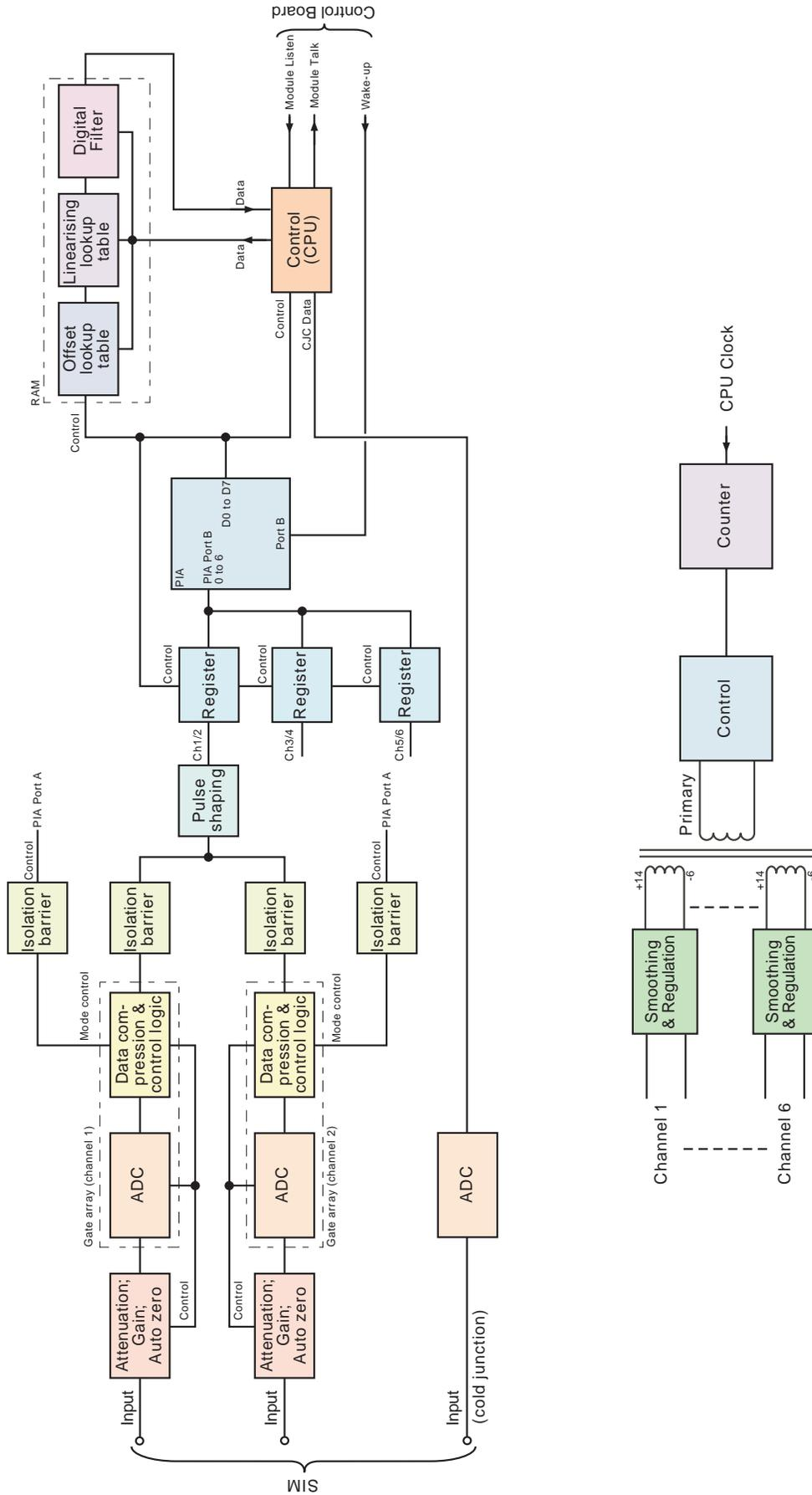
Figure 2.1 DC input board - block diagram
