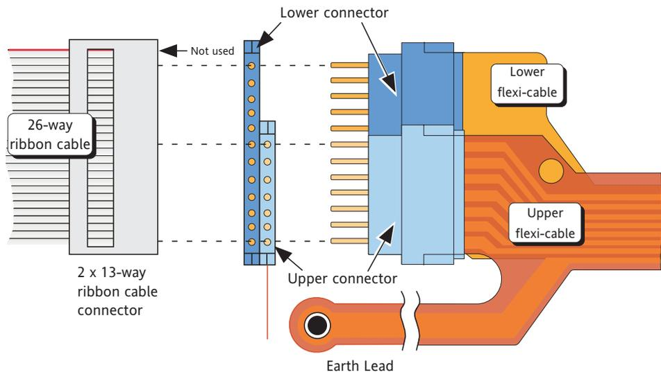
Figure 5.2.4 Print head carriage flexi-cable connectors
