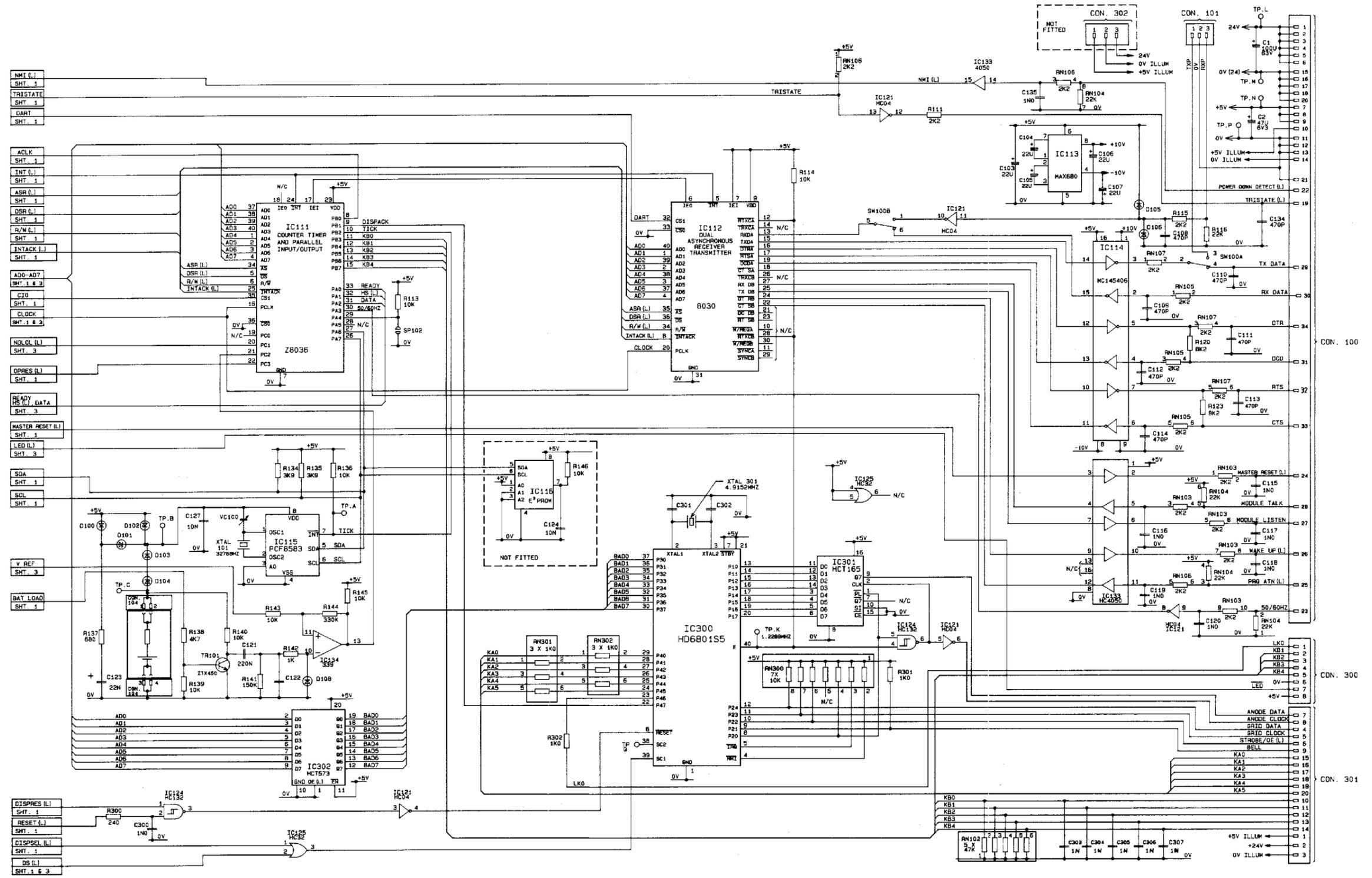
Figure 6.9.2b Mark II Control board schematic (sheet 2)
