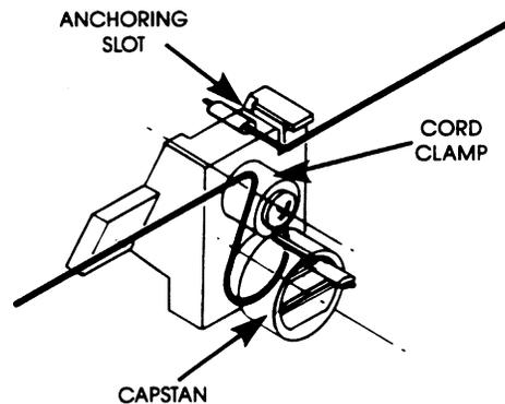
Figure 5.4.7b Cord anchoring
