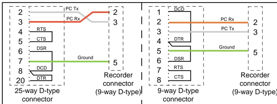
Figure 1.6b Configuration transfer port to host computer wiring
