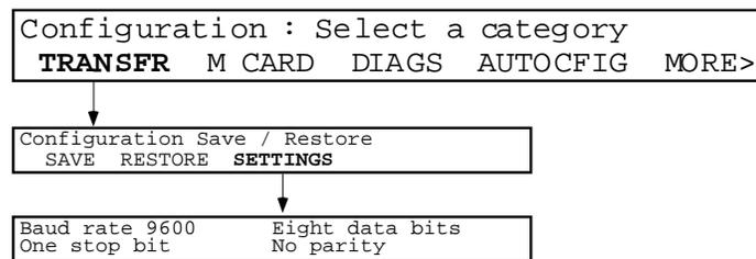
Figure 4.10 Configuration-transfer configuration
