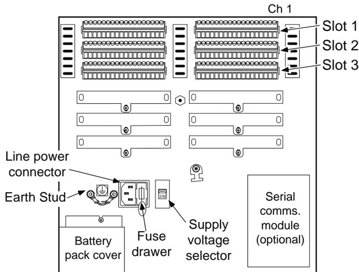
Figure 1.4.1 Recorder rear view with terminal cover removed
