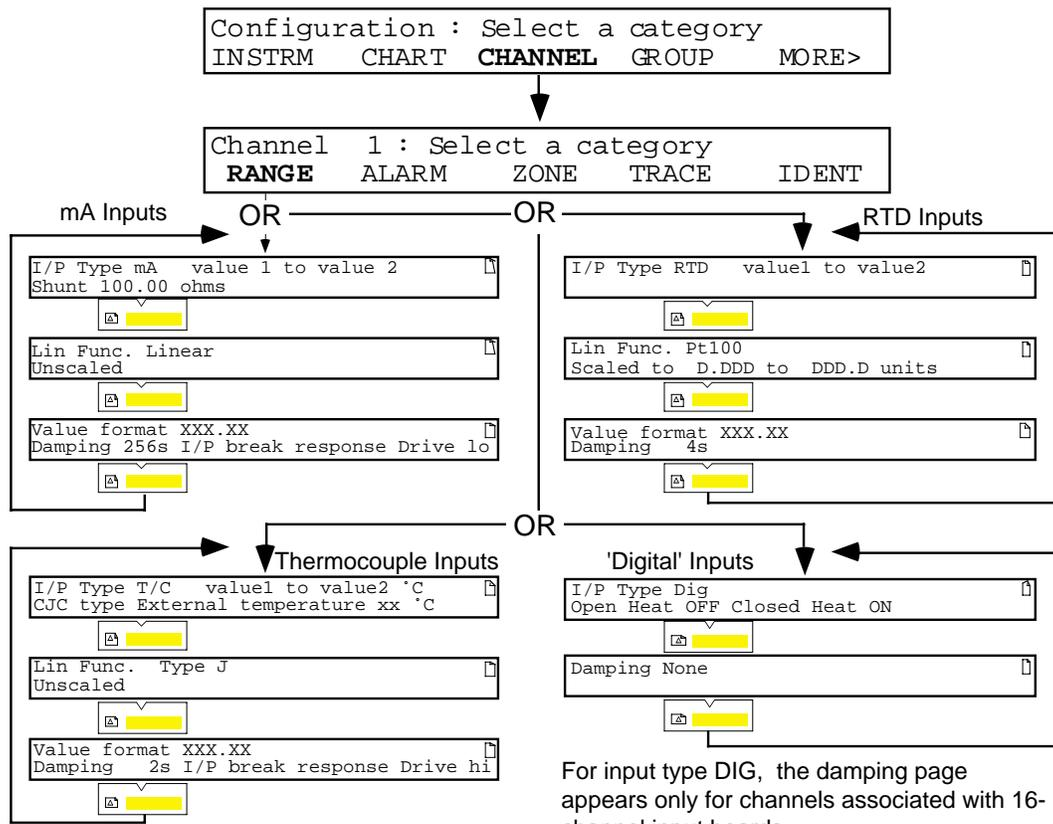
Figure 4.4.2a input channel configuration: Typical range pages
