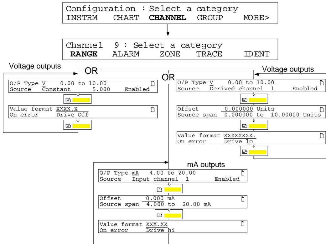
Figure 4.4.2b Output channel configuration: Typical range pages
