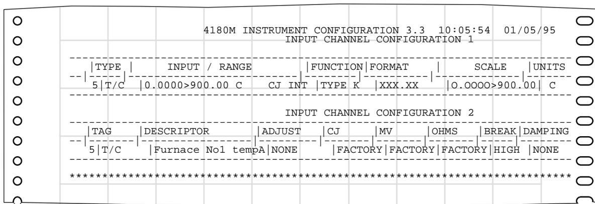
Figure 2.3.1 Channel configuration printout
