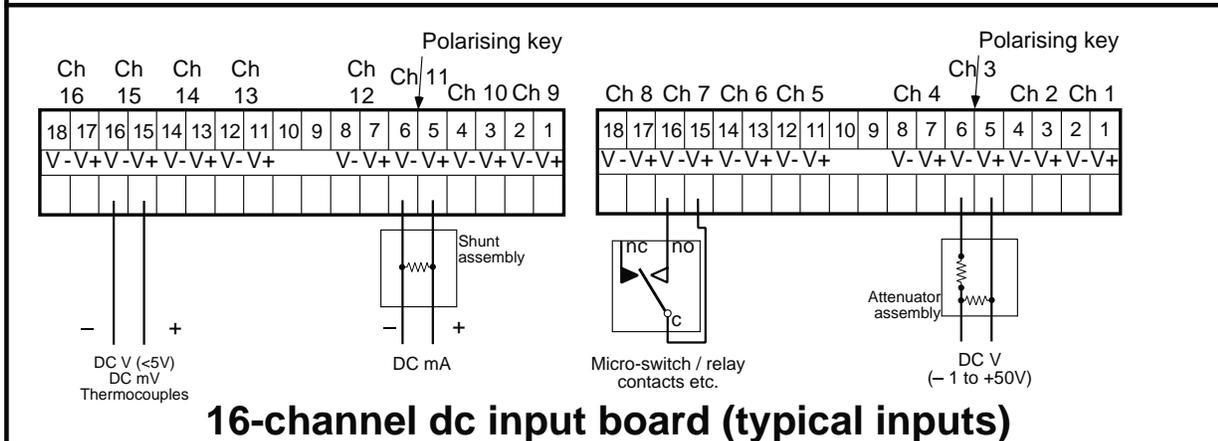
Shunt part n s: 100 = LA246779UK10; 250 = LA246779UK25. Attenuator part n = LA244180U100
