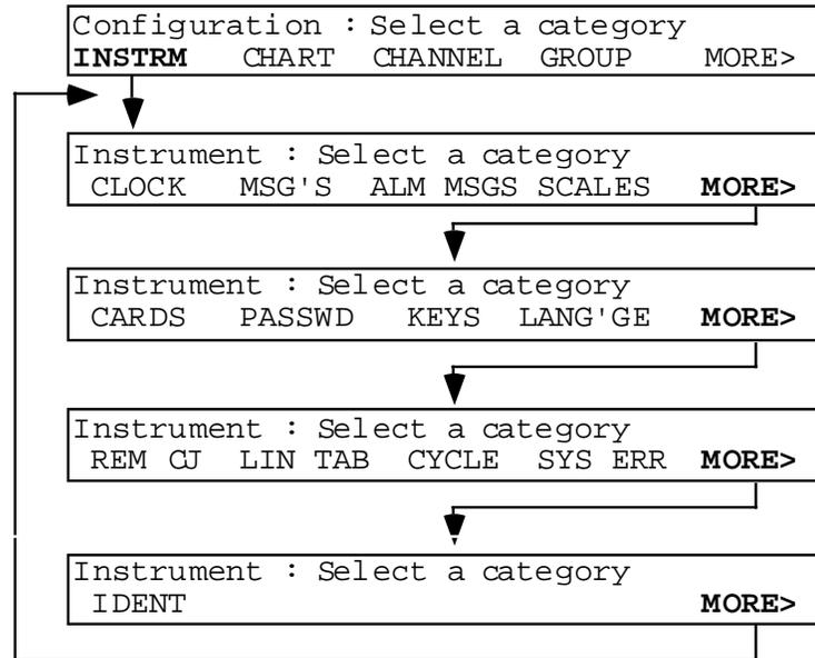
Figure 4.2 Instrument configuration
