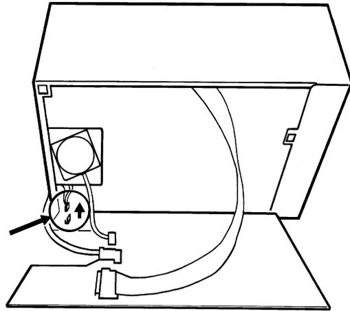
Figure 4.9b Chart drive motor disconnection
