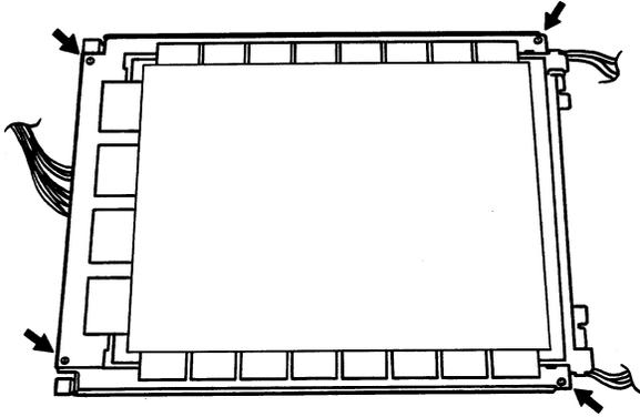
Figure C1.4c Display removal (3)
