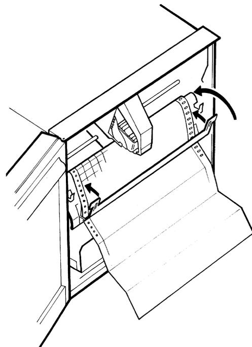
Figure 2.1.1d Z-fold chart loading (2)
