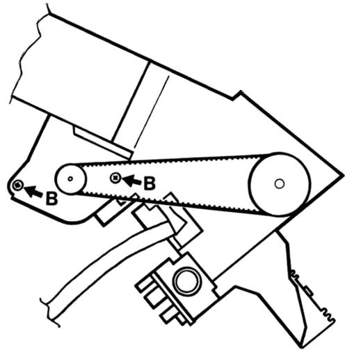
Figure 4.4b Ribbon motor securing screws
