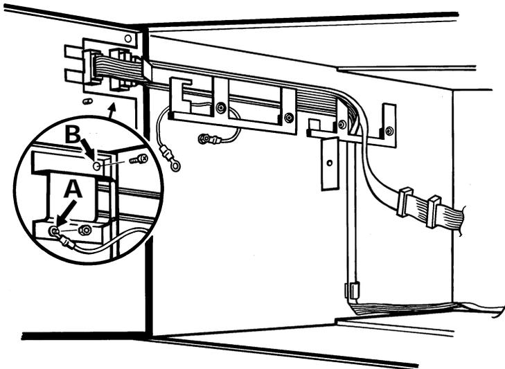
Figure C1.2a Earth lead and cover removal
