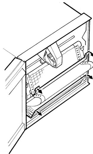
Figure 2.1.1a Z-fold chart removal
