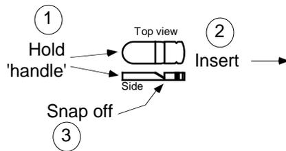
Figure 4.14d Polarising key fitting
