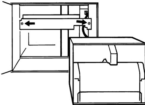
Figure 4.2c PCB retainer securing screws
