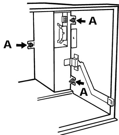
Figure 4.11.3b PSU removal
