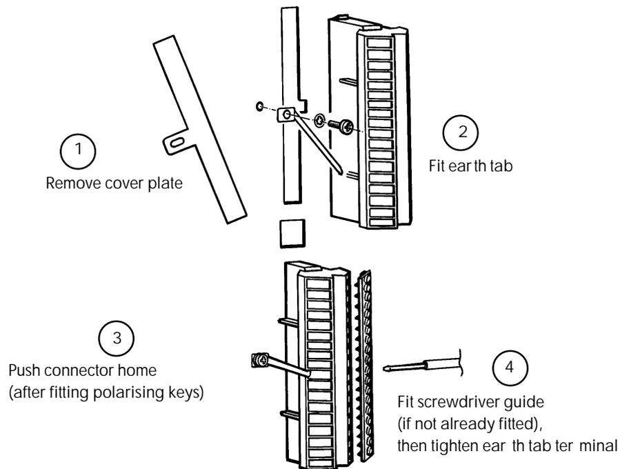
Figure 4.14b Connector installation
