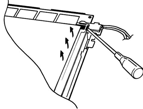
Figure C1.4d Release of backlight securing plate
