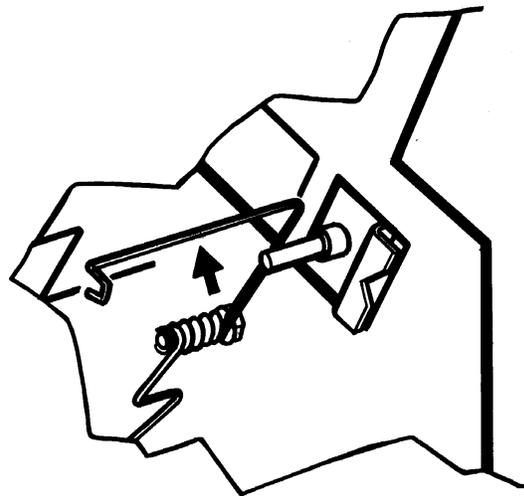
Figure 4.8c Paper-out detector actuator
