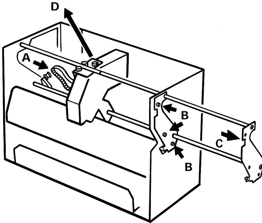
Figure 4.3d Printhead carriage removal
