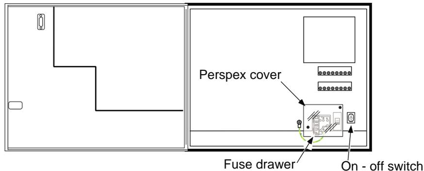
Figure 3.1.1c On-off switch and supply voltage components for Graphics Display Units
