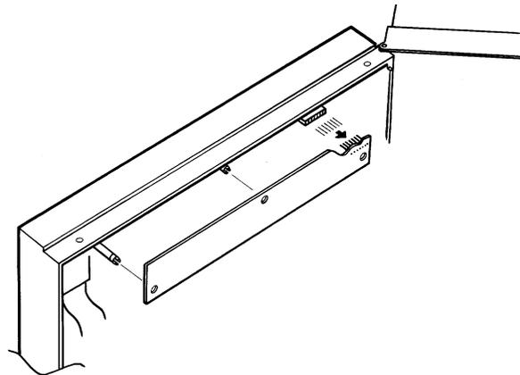
Figure 4.12.3b Electrical connections
