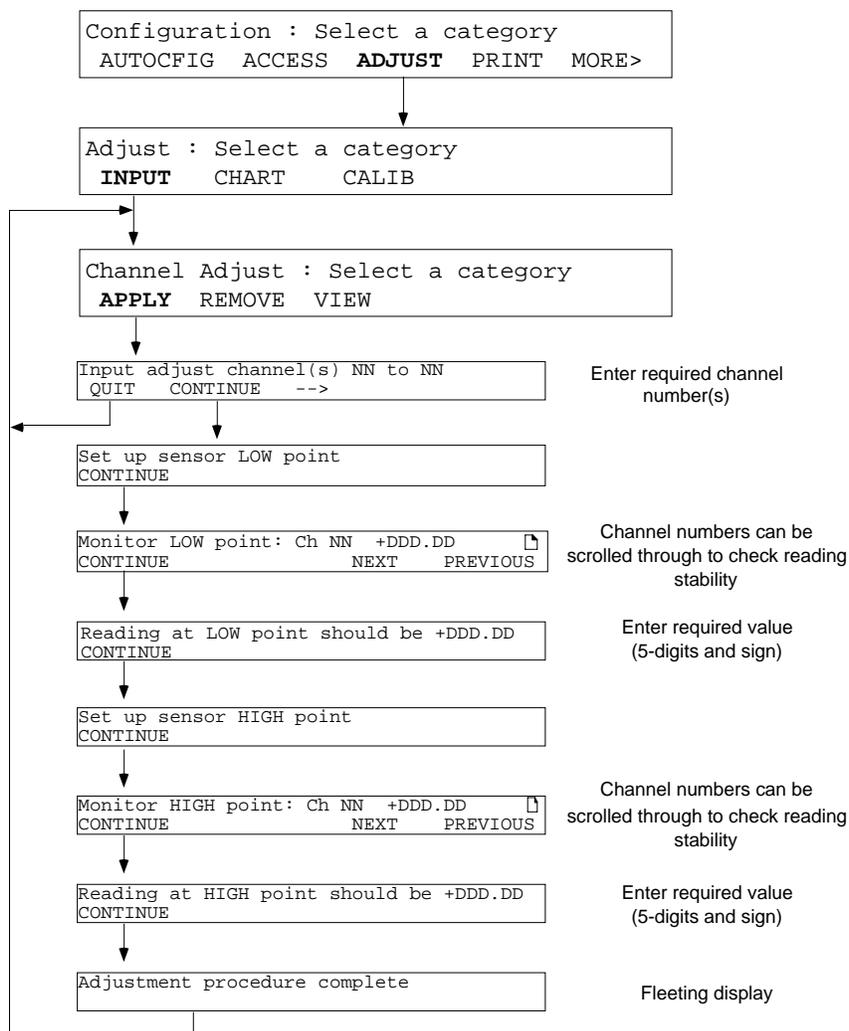
Figure 3.4.1 Channel Input Adjust menu
