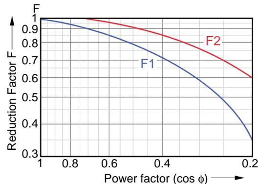
Figure 1.2.4 Reduction factor for inductive loads
