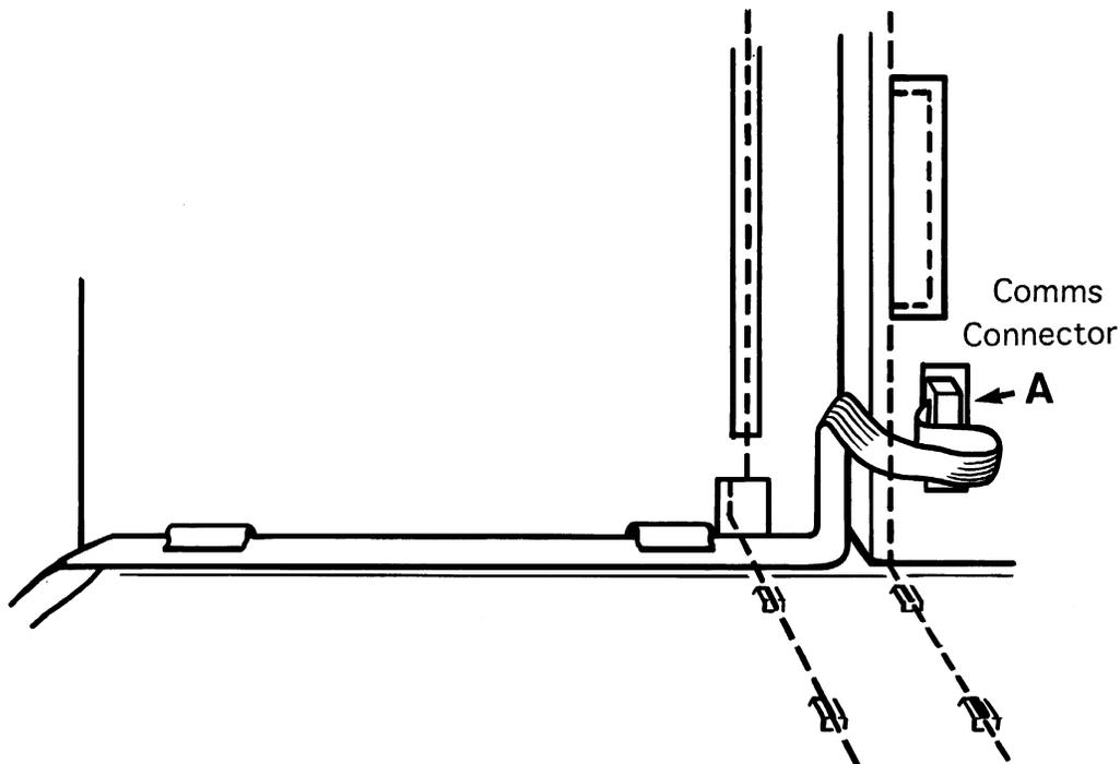
Figure C3a Comms connector location (view on inside of case)
