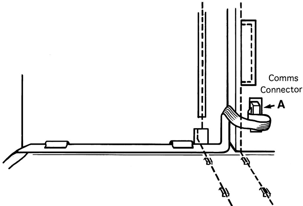
Figure 4.13.2a Comms connector location (view on inside of case)
