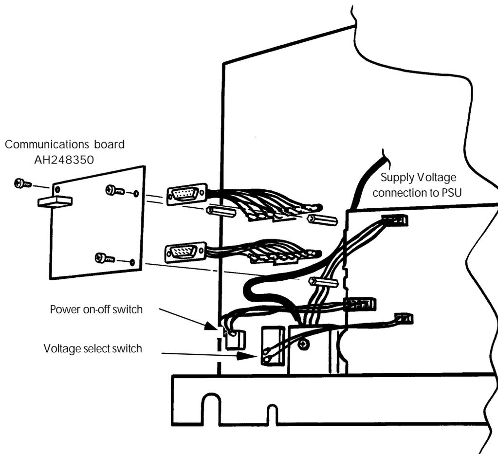
Figure A1.2c Communications board and power connections
