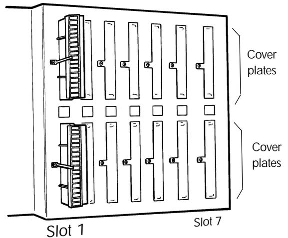
Figure 4.14a Rear view with terminal cover removed
