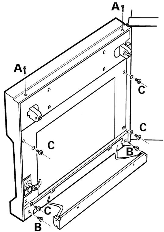
Figure 4.12.2 Inner door cover removal
