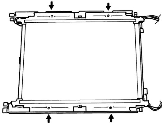
Figure C1.4e Securing plate removal
