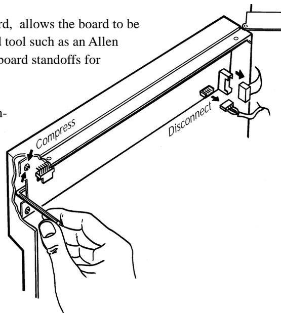
Figure 4.12.5 Display board removal
