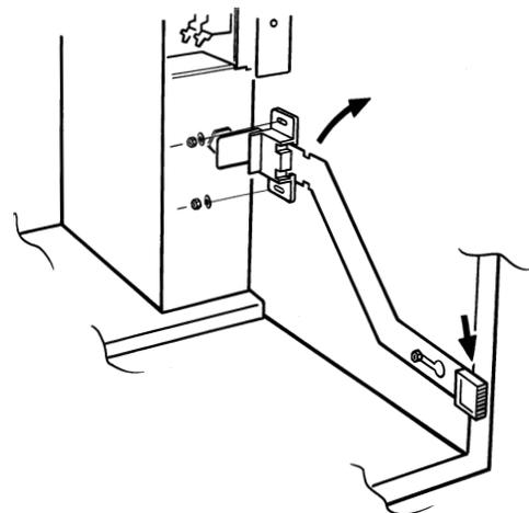
Figure 4.11.4 On-off switch removal
