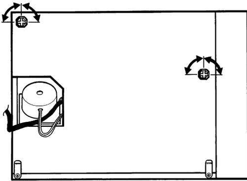
Figure 4.9a Writing system circuit board release
