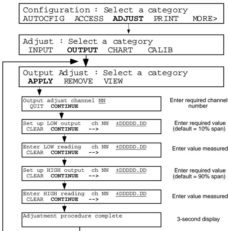
Figure 3.4.2 Output channel adjust menu
