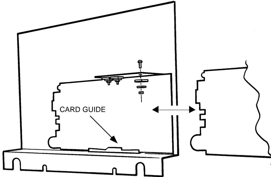
Figure A1.2a Power supply securing
