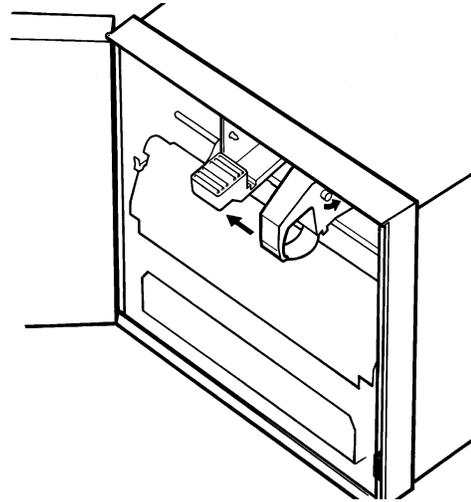
Figure 2.2 Ribbon cartridge replacement
