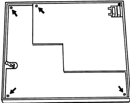
Figure C1.3a Inner cover securing screws
