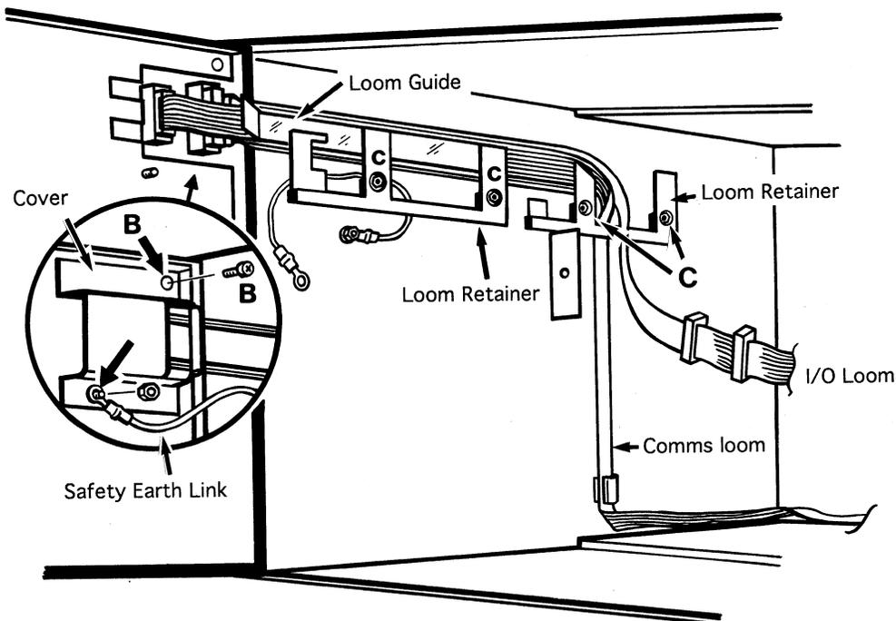
Figure C3b Loom replacement
