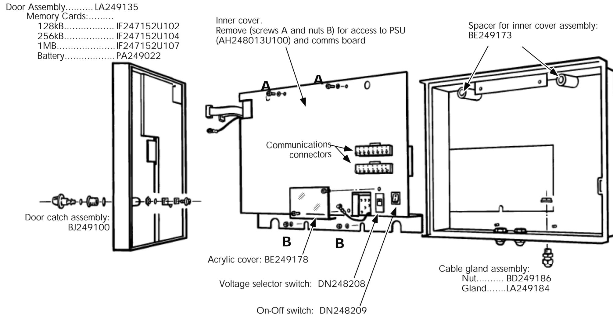
Figure A1 Graphics display Unit exploded diagram
