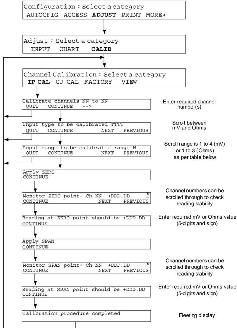
Figure 3.4.4 Input channel calibration menu
