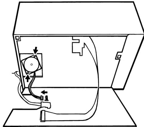
Figure 4.7.1b Printhead carriage motor
