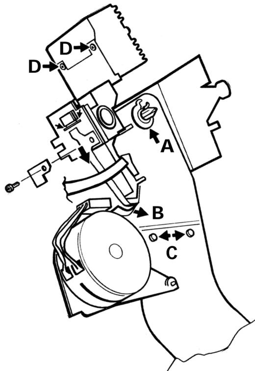
Figure 4.6 Printhead replacement
