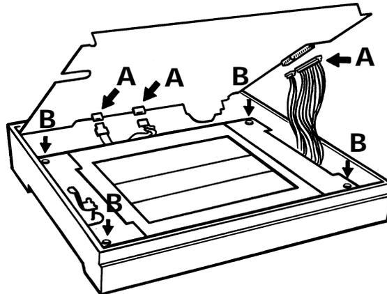
Figure C1.3b Inner cover removal
