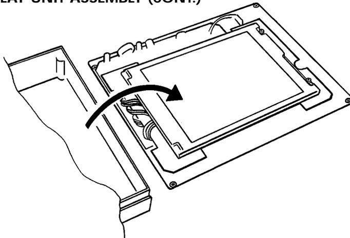
Figure 4.13.1 f Display unit removal
