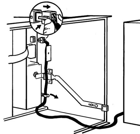
Figure 4.2d PSU connector release
