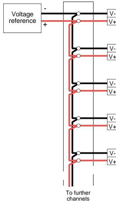
Figure 3.2.2 DC Calibration check wiring (16-channel input board)
