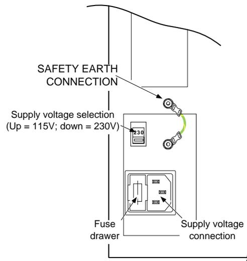
Figure 3.1.1b Supply voltage components (Recorders)
