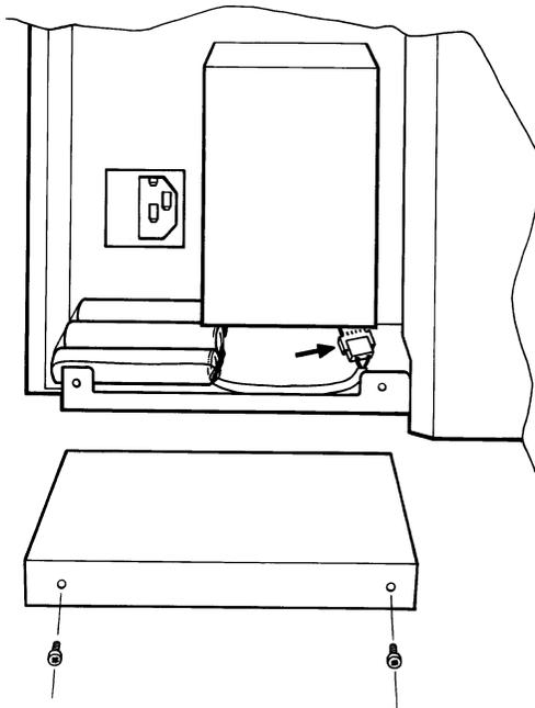
Figure 4.15.1 Recorder battery replacement
