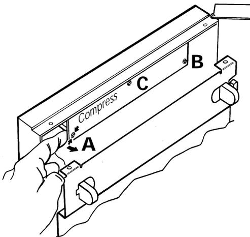
Figure 4.12.3a High-voltage board release
