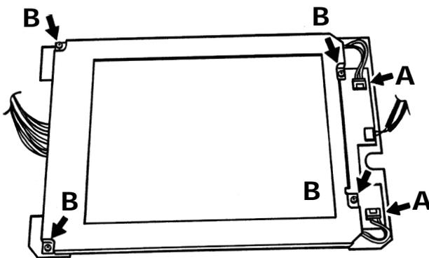
Figure C1.4a Display removal (1)
