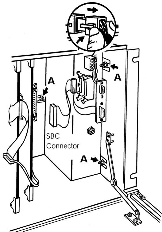
Figure B.2b Power Supply removal
