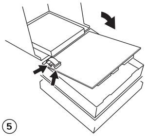
Rotate the cover downwards, at the same time allowing the microboard to move forwards. Disconnect the touch panel flexi-cables.
