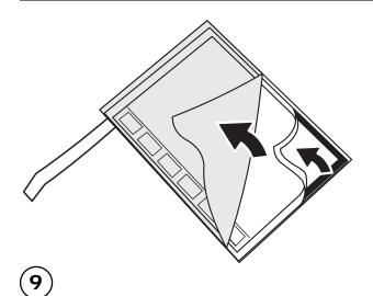
Remove the protective sheet from the front of the screen.
