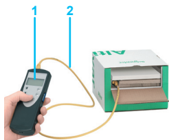
Configuring the drive in its packaging with the Multi-Loader tool VW3A8121+ cordset VW3A8126
