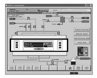
During this cycle, accurate temperature control is important and a heating jacket is used. As the overall duration of this cycle is around 60 hours, high availability of the system is vital and system redundancy is required. Doubling sensors, actuators and controllers as well as changeover facilities on these components, helps to ensure the product is sterilised even on hardware or software failure.
