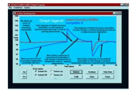
Testing Action's temperature transmitter by introducing a 25 degree C thermal plunge resulted in the following: the peak excursion was 1.15 degrees C but settled within 15 minutes at the final offset value of 0.6 degrees C.
