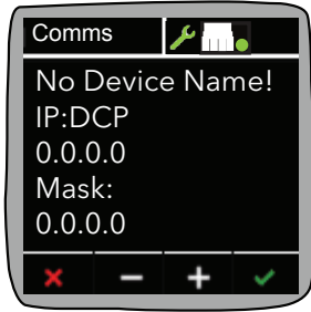
Figure 39 EPack 'Comms' screen display 'as-delivered' (Device Name = "", IP Configuration = Null).
