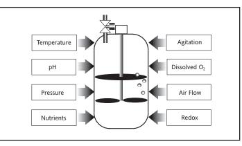
Temperature, pH,  $DO_2$  or Redox, agitation, pressure, foam control, auxiliary feed or a combination of these controllers.
