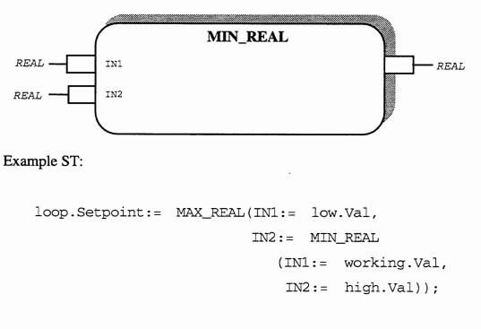
loop.Setpoint is set to working.Val limited between a minimum set by low.Val and a maximum set by high.Val.
