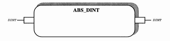
Functions have a single output which is shown on the right-hand side of the diagram.
