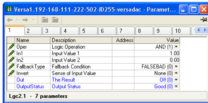
Figure 110 Two-input logic block configuration
