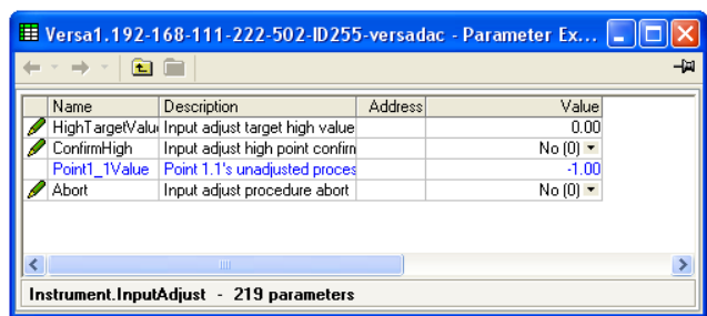
Figure 68 Input adjust High and Low targets
