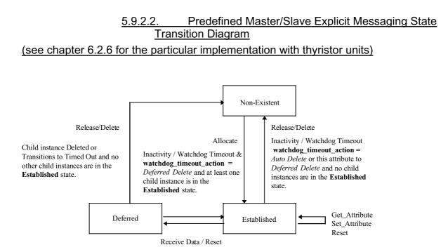
The SEM presented above provides a formal definition of the behaviour of the Explicit Messaging Connection within the Predefined Master/Slave Connection Set. This SEM inherits from and/or overrides actions presented in the Explicit Messaging Connection Object SEM.
