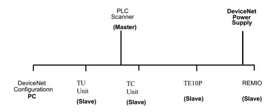
Many of the steps involved in the creation and configuration of an Application to Application connection have been removed within the Predefined Master/Slave Connection Set definition.
