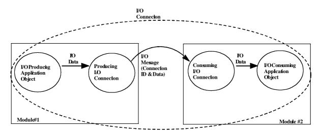
The Specification does not define any particular use for I/O Messaging. There are a wide variety of functions that can be accomplished using I/O Messaging.
