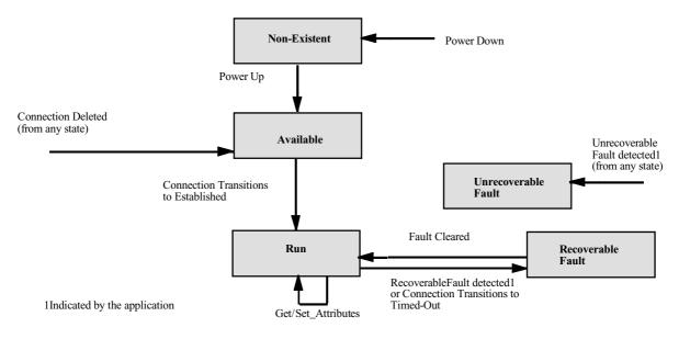
Important: Events can occur simultaneously, but the Fault events have priority if they occur simultaneously with other events.
