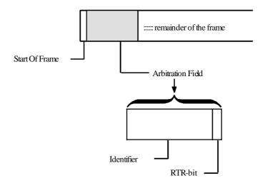
The 11\_bit Identifier Field is transmitted from most significant to least significant bit. A bit on the bus can be either dominant (value 0) or recessive (value 1). Simultaneous transmission of a dominant bit and a recessive bit results in the presence of a dominant bit. Refer to section 9-1.3 vol. 1 of the DN specifications for information concerning DeviceNet s representation of the dominant and recessive levels.
