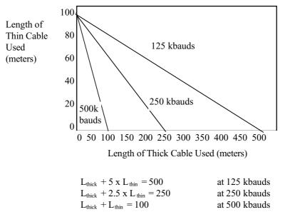
where  $L_{\text{thick}}$  is the length of thick cable and Lthin is the length of thin cable.
