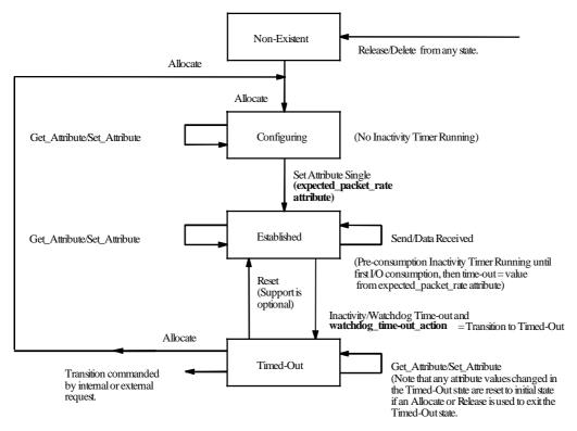
Note that the Allocate and Release services send the connection instance back to initial state. All Object attributes are reset to their default values.
