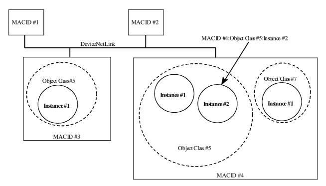
It is also possible to address the Class itself versus a specific Object Instance within the Class. This is accomplished by utilising the Instance ID value zero (0). DeviceNet reserves the Instance ID value zero (0) to indicate a reference to the Class versus a specific Instance within the Class.
