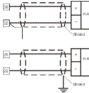
Fig. 6A – 6 mA INPUT WIRING
