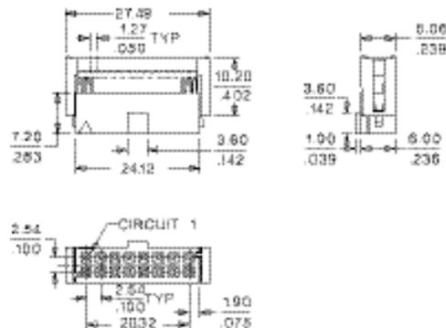
Fig. 15 – CONNECTOR 8x2 FOR BUS CABLE
