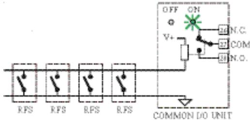
Fig. 20A – Relay de-energized, beacon ON lit.
