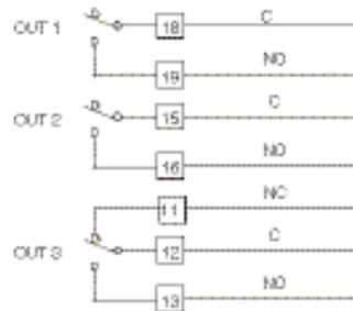
Fig. 9 – RELAY OUTPUTS WIRING
