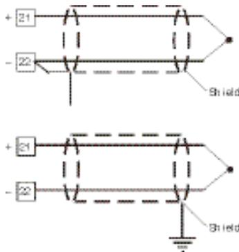
Fig. 4 – THERMOCOUPLE INPUT WIRING
