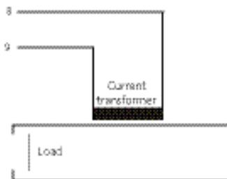
Fig. 8 – CURRENT TRANSFORMER INPUT WIRING
