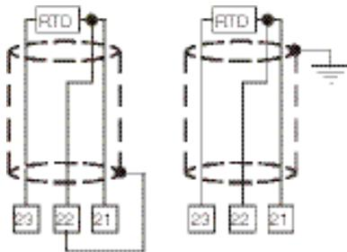
Fig. 5 – RTD INPUT WIRING
