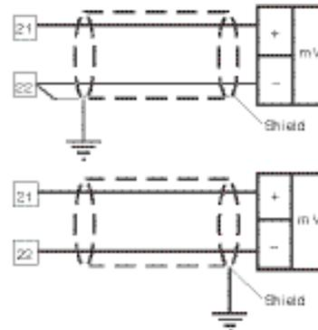
Fig. 6B – 60mV INPUT WIRING
