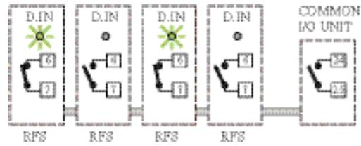
Fig. 18A - Common logic input OPEN
