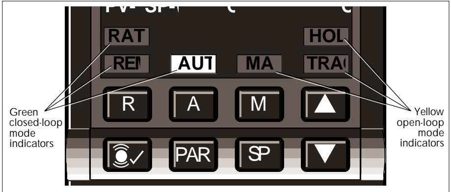
Figure 3-7 Operating mode indicators — example showing Auto(matic) mode operating
