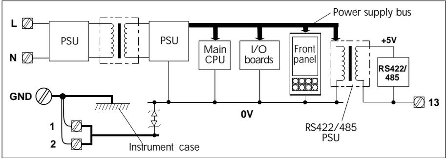
Figure 2-7 T640 internal zero volts & power supplies schematic
