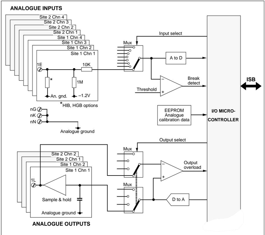
Figure 11-2 Analogue input & output block schematic
