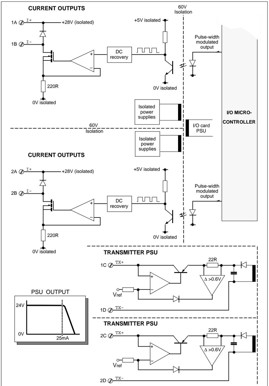
Figure 11-4 Current output & transmitter PSU block schematic
