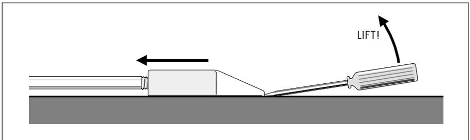
Figure 2-3 Removing a clamp from the sleeve
