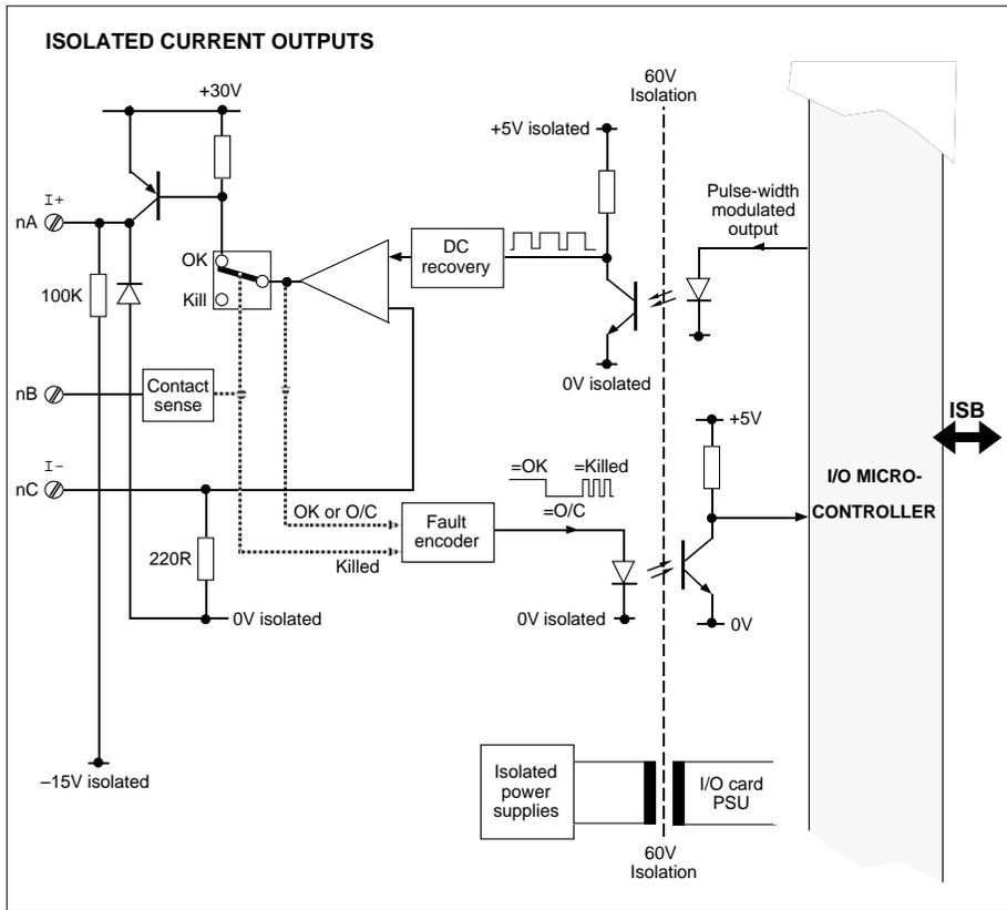
Figure 11-10 Isolated current output block schematic (n=1, 2)
