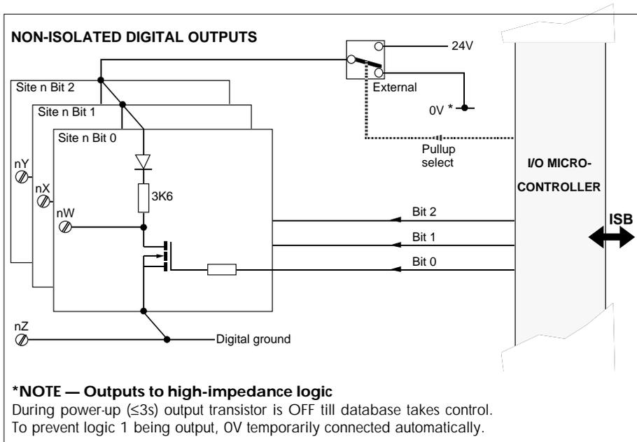
Figure 11-12 Non-isolated digital outputs block schematic (n=1, 2)
