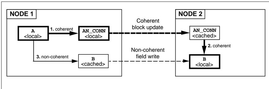
Figure 8-1 Coherent & non-coherent data flow across the network
