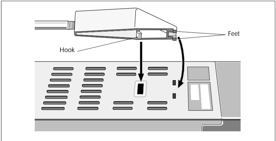
Figure 2-2 Fitting a clamp to the sleeve
