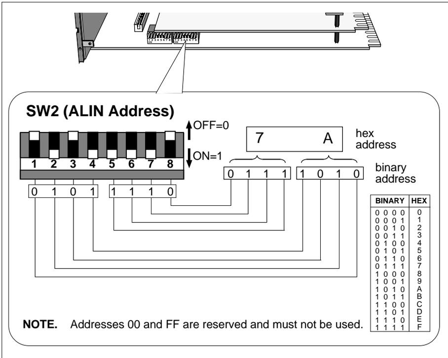
Figure 2-13 SW2 — ALIN address setup (example)
