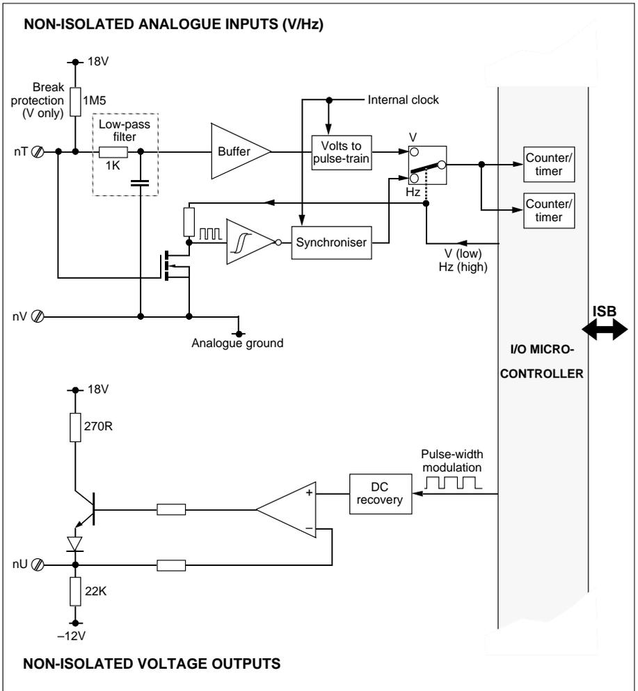
Figure 11-9 Non-isolated analogue input/output block schematic (n=1, 2)
