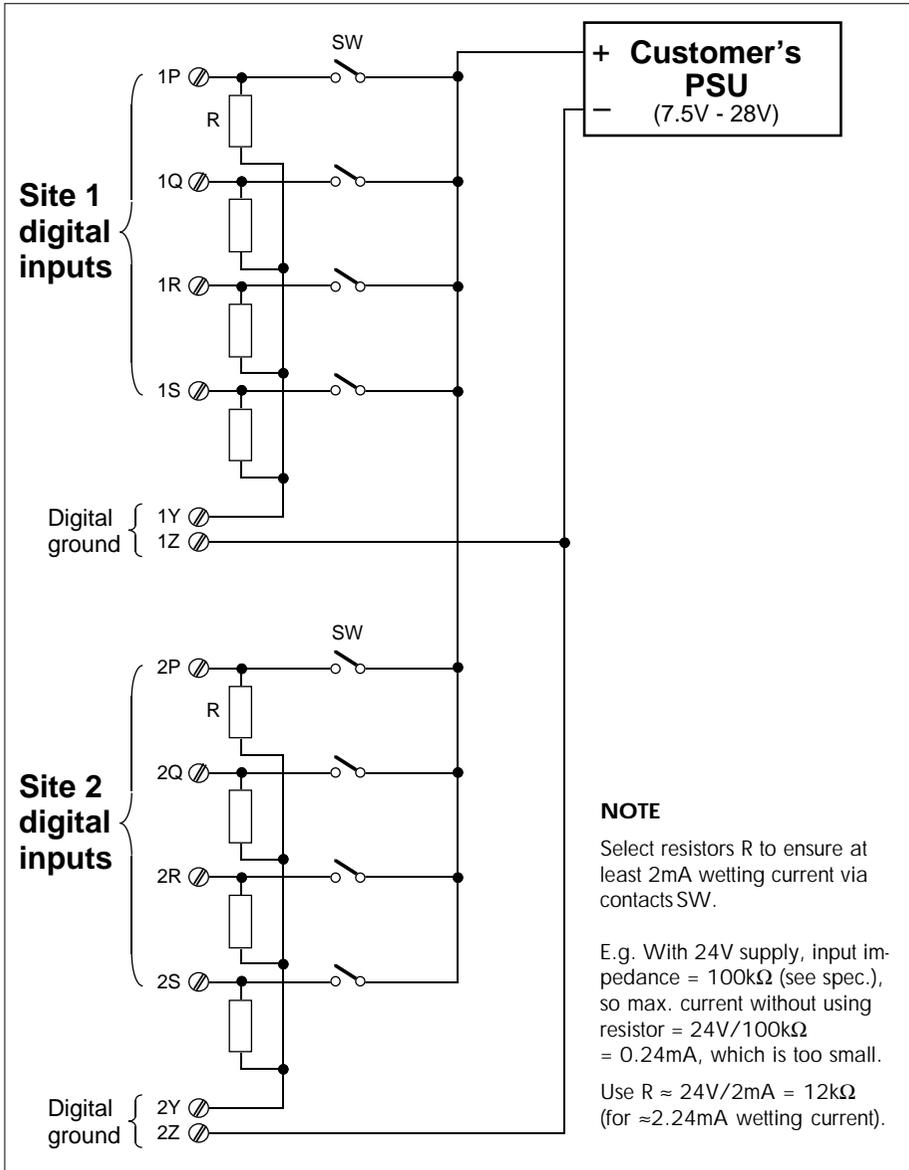
Figure 11-7 Digital input contact-sensing using customer's PSU
