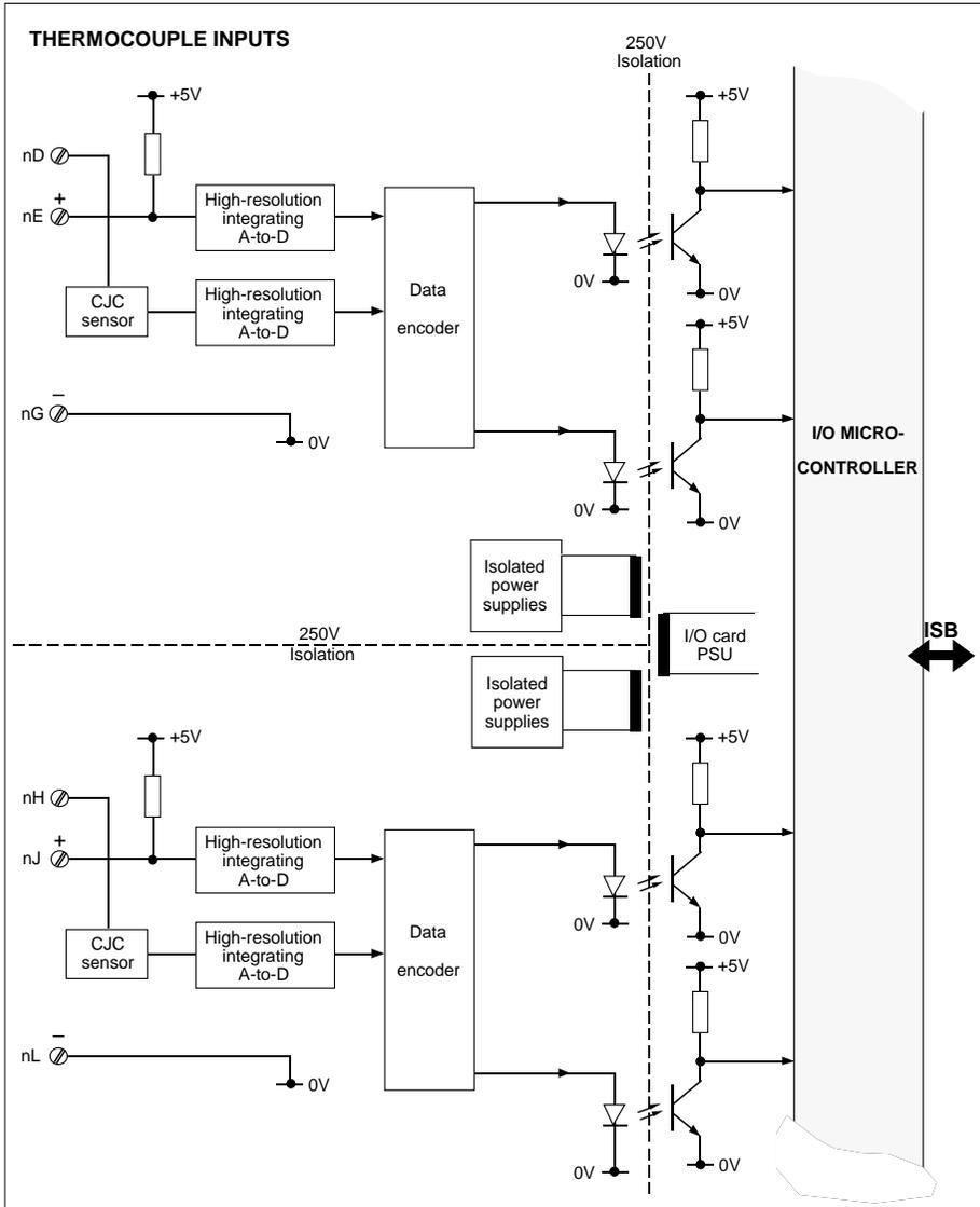
Figure 11-8 Thermocouple inputs block schematic (n=1, 2)
