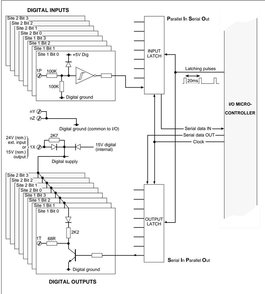
Figure 11-3 Digital input & output block schematic
