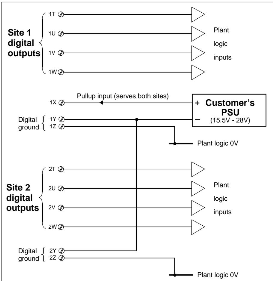
Figure 11-5 Digital outputs driving plant logic using customer's PSU
