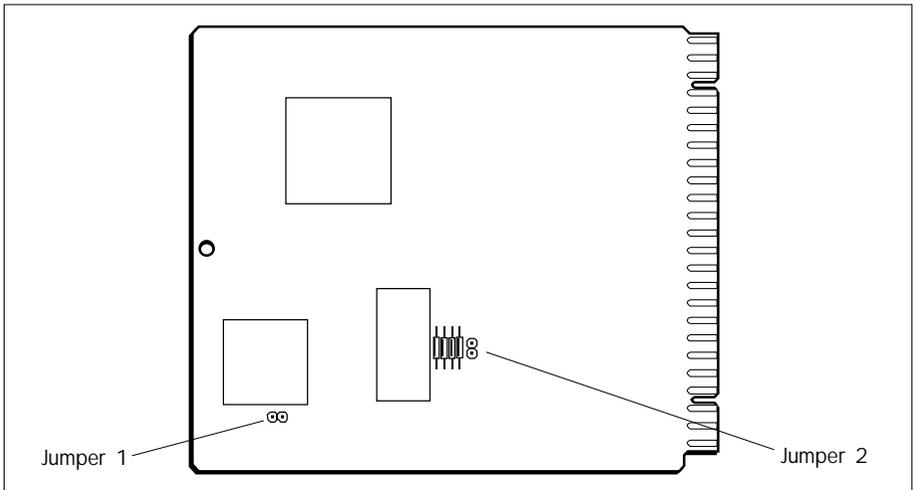
Figure 11-1 High-level I/O board showing 0 - 1.25V range jumpers
