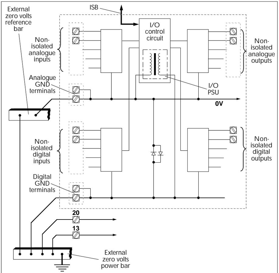
Figure 2-8 T640 I/O zero volts & power supplies schematic
