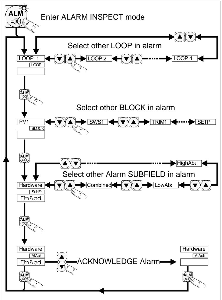
Figure 3-8 Alarm inspect button functions — ALM
