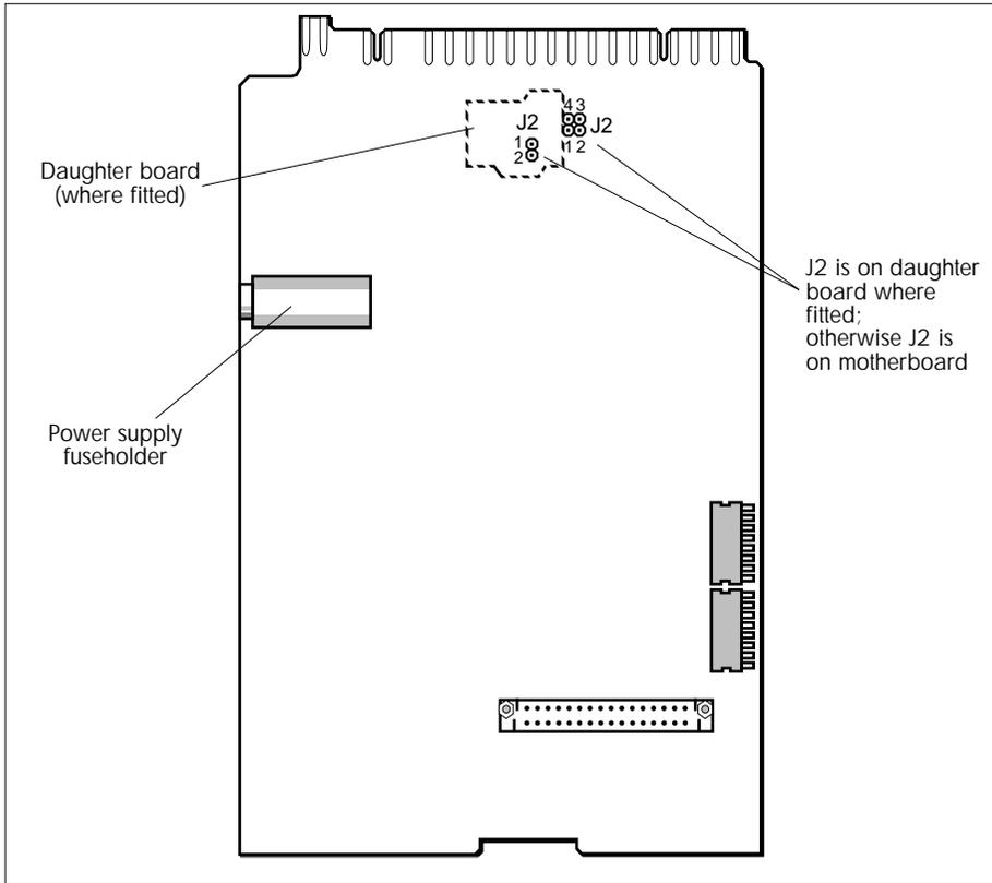
Figure 2-11 T640 motherboard showing fuse & jumper locations
