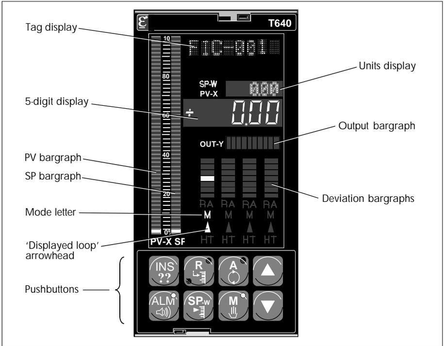
Figure 2-16 T640 front panel — principal features
