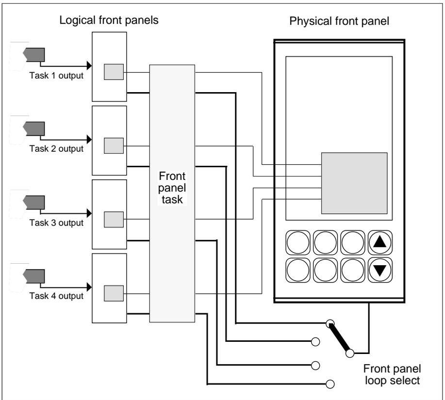
Figure 7-2 T640's logical & physical front panels
