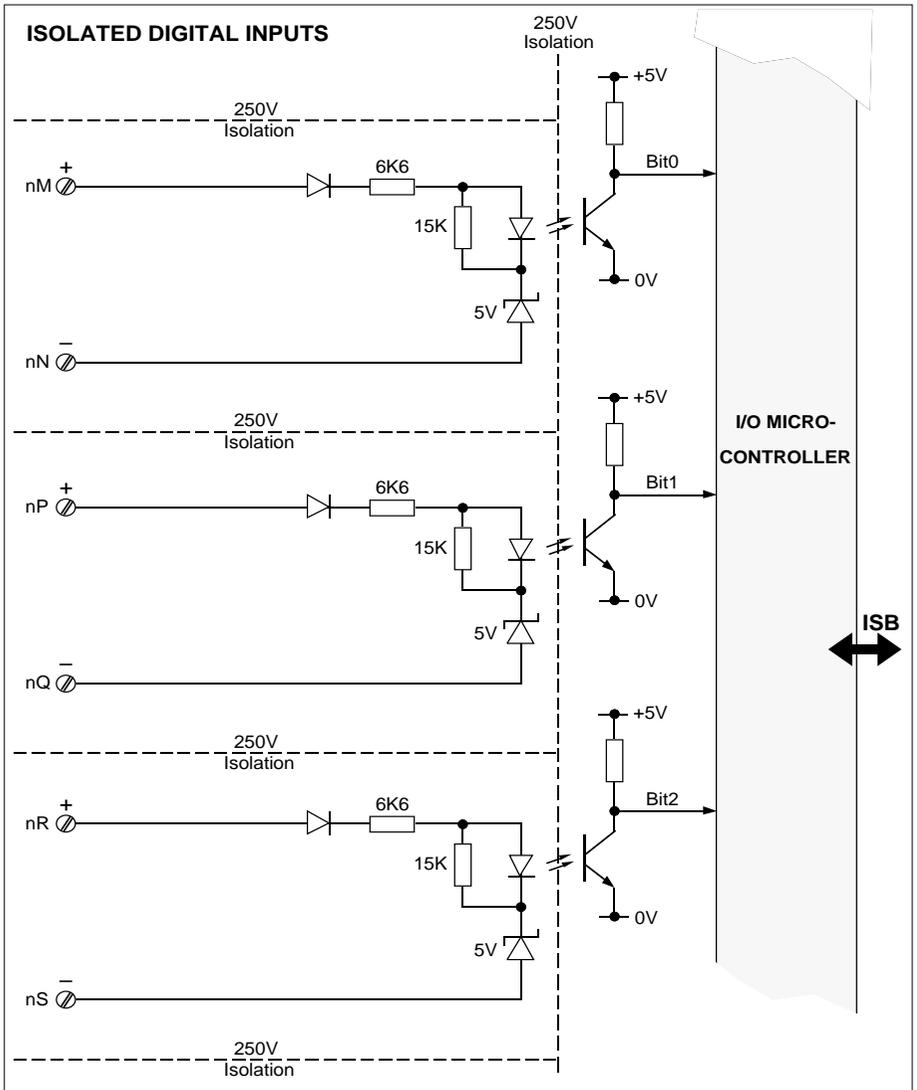
Figure 11-11 Isolated digital inputs block schematic (n=1, 2)
