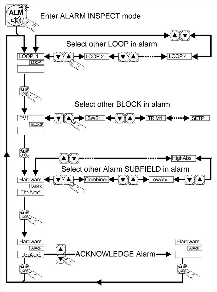
Figure 4-3 Alarm inspect button functions — ALM
