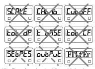
Figure 17. Functions Locked Out with Lockout Jumper
