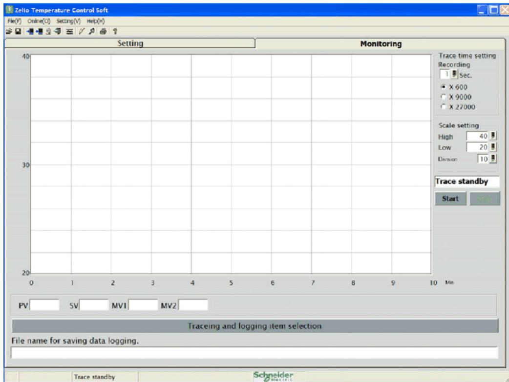
When tracing is stopped, press the Trace icon on the tool bar or click **Online(O) → Trace(T)** on the menu to start tracing (logging).
