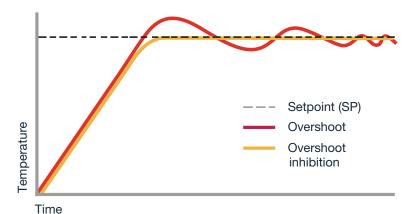
Eurotherm cutback and over-ramp suppression functions significantly minimize overshoot and instability, reducing the risk of over or under-heating workpieces. They also help to optimize energy usage and minimize production time and waste
