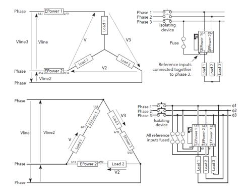
However, the above requirements are not needed to control certain types of applications, such as SiC element-based tin bath roof heating systems in the glass industry. This was one of the most important types of application considered by Eurotherm during the design of the EPower range in terms of possible efficiency improvements, and it resulted in the recommendation of using two leg burst firing control either in star or delta configuration, as in Figure 3 and Figure 4.
