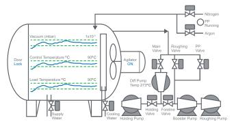
Typical vacuum furnace layout, visualized in E+PLC
